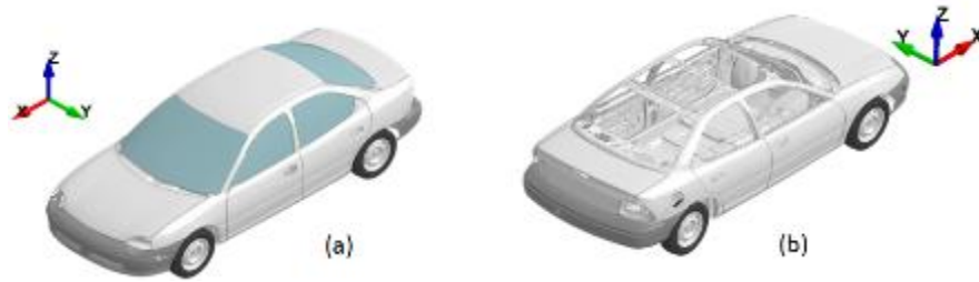
Figure 2.1 (a) 1996 Dodge Neon Model by NCAC with (b) roof, windshields and side windows removed to reveal the lack of any interior component.
