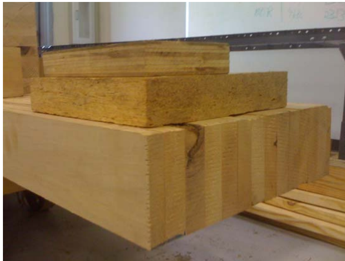
Figure 2.1 Examples of Structural Composite Lumber - LVL, OSB, Glulam
