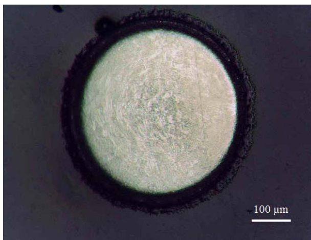
Figure 2.8 An optical micrograph of unannealed Pt substrate #W electrode after 75 s electrolytic etching in etching solution #1.
