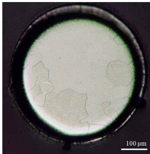
Figure 4.7 Optical micrograph of an etched polycrystalline Pt substrate (Sub #J).
