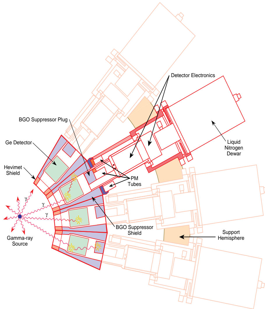
Figure 4.3: Gammasphere Detector Geometry [71].
