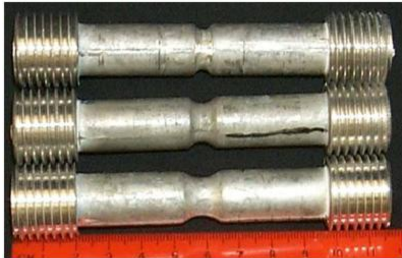
Figure 2.1 Three AM60B magnesium notched Bridgeman tensile specimens with three different notch geometries. The geometry used in this study is series H, the top specimen, with a notch radius of 0.635 cm.
