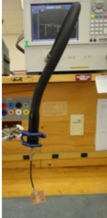
Figure 11 Set Up For Agilent Network Analyzer Measuring Return Loss.
