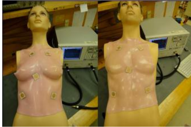
Figure 17 Female and Male Mannequins with Skin Layer and Antennas in Place
