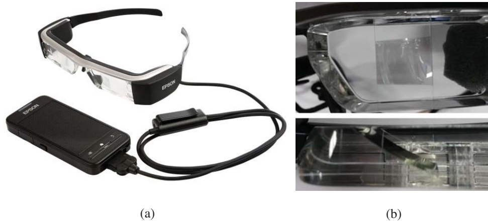
Figure 2.4 OST HMD with partially silvered mirror combiner
