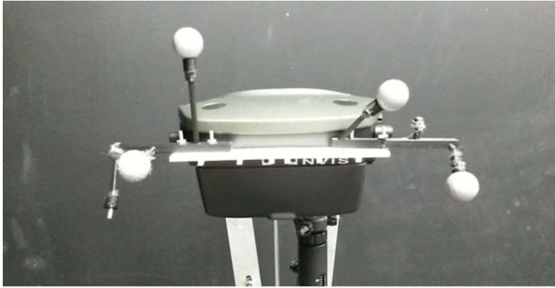
Figure 4.23 ST50 HMD with retro-reflective constellation
