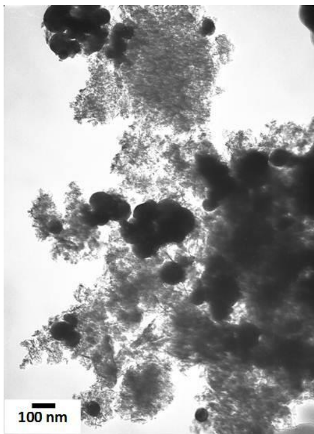
Figure 3.8 TEM image of 3D asymmetric Janus magnetic nanoparticles deposited from isopropanol
