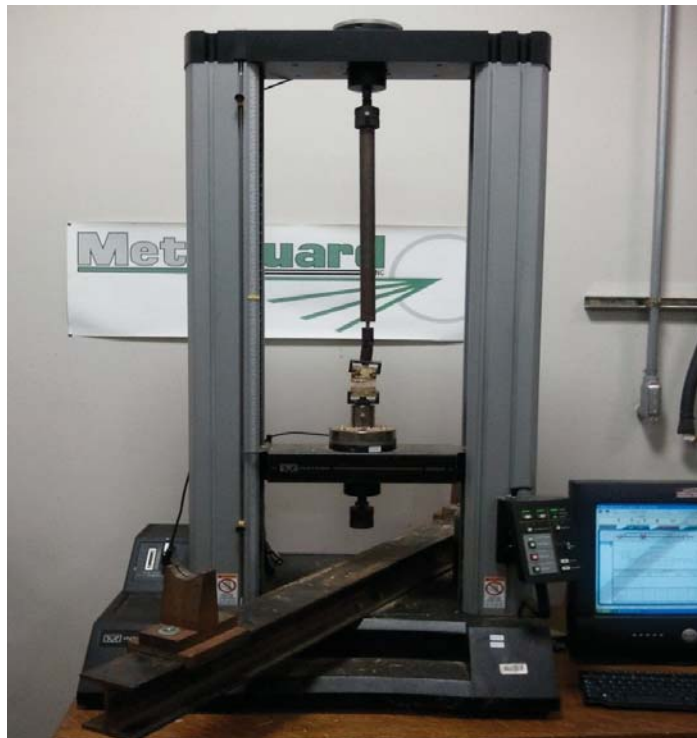
Figure 2.21 Internal bond test
