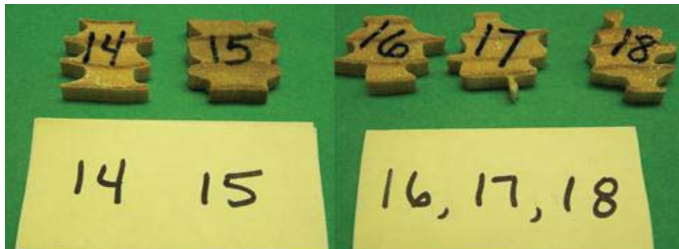
Figure 3.25 Block appearance for southern pine positive control after 28-day termite test
