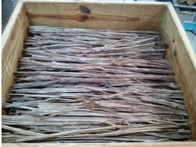
Figure 2.9 Forming box used in scrim layup
