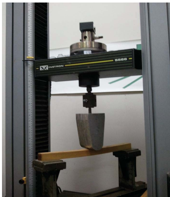
Figure 2.30 Bending test-center point loading
