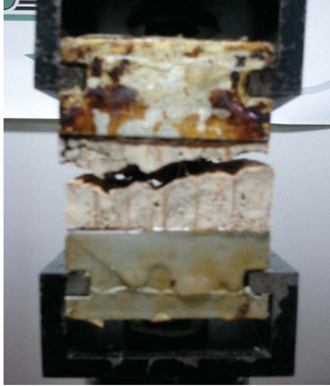
Figure 3.2 Typical rupture failure for IB test
