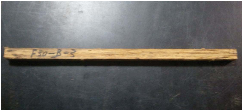
Figure 3.10 Sample treated with 30% FA after tension failure (Looks intact outside, inside layer broken)
