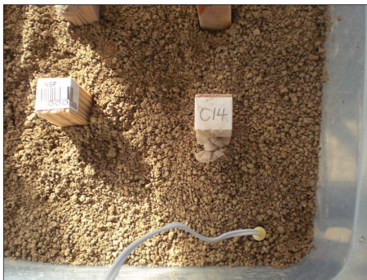
Figure 2.2. Monitoring of control wood stakes during soil bed decay test. Temperature, humidity, and moisture content were monitored during decay test. The sensor detects temperature and humidity in the container. Wood stakes with nylon stocking material were used to monitor the moisture content of wood stakes.
