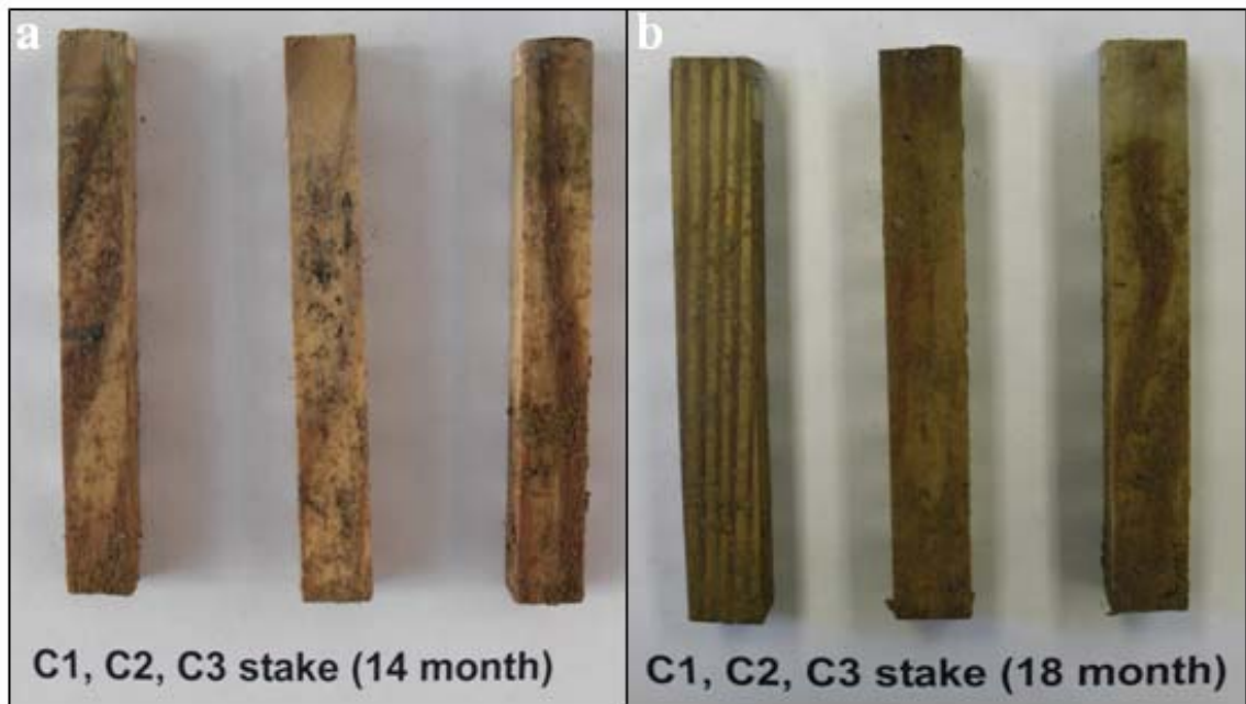
Figure 2.24. Visual observation of ACQ-treated pine wood stakes (a) at 14 months and (b) at 18 months.
