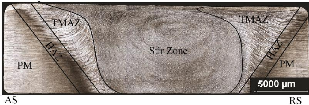
Figure 3.2 Transverse view of a conventional FSW with regions of interest labeled.
