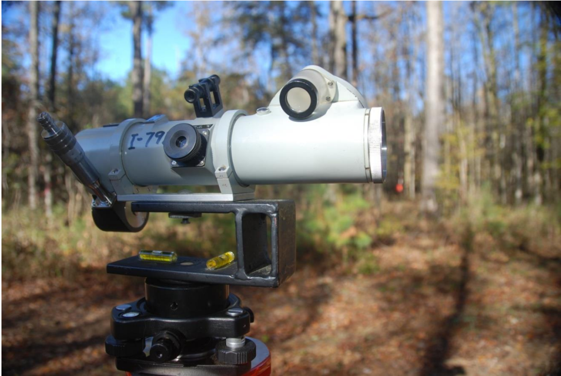
Figure A.2 Barr & Stroud FP15 optical dendrometer.
