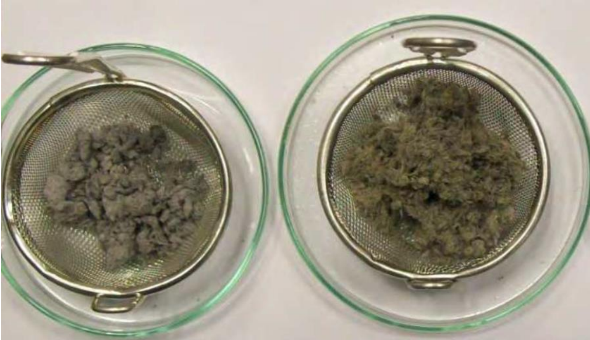
Figure 5.5 Paper mill sludge (PMS); (left) raw PMS, (right) unraveled PMS
