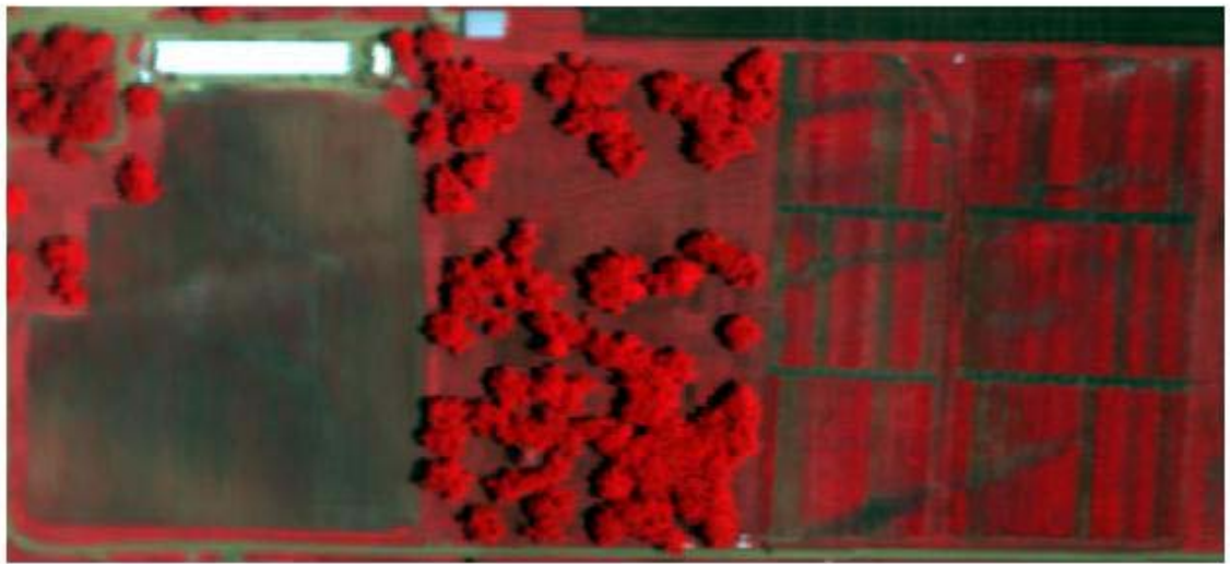
Figure 1.2 Optical remote sensing – Top: RGB true color composite with Blue-488nm, Green-533nm and Red-602nm. Top: RGB false color composite with Blue-533nm, Green-602nm and Red-753nm. Both show hyperspectral image of Mississippi State fields at Brooksville, MS, acquired using an airborne SpecTIR™ inc. sensor.
