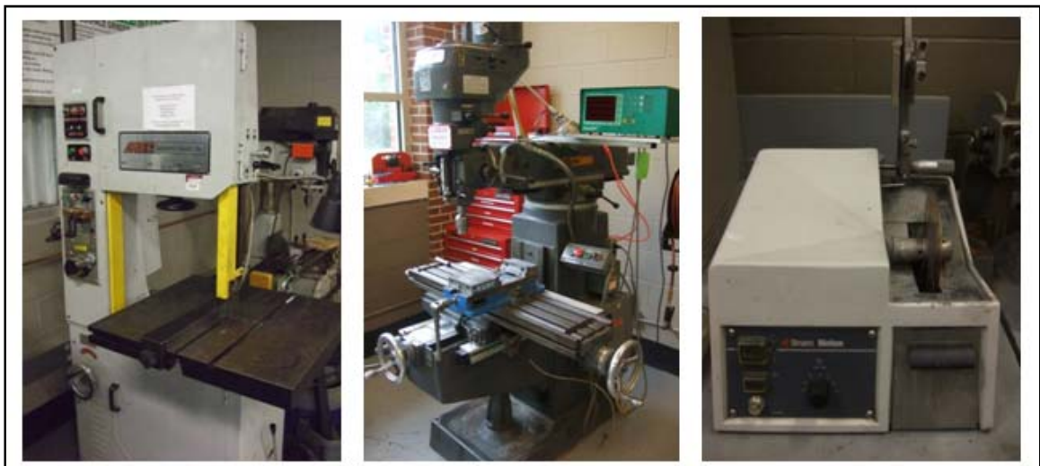
Figure 3.1 The machining tools used to prepare samples from the rolled sheet for channel die compression. From left to right: band saw, mill, diamond saw.
