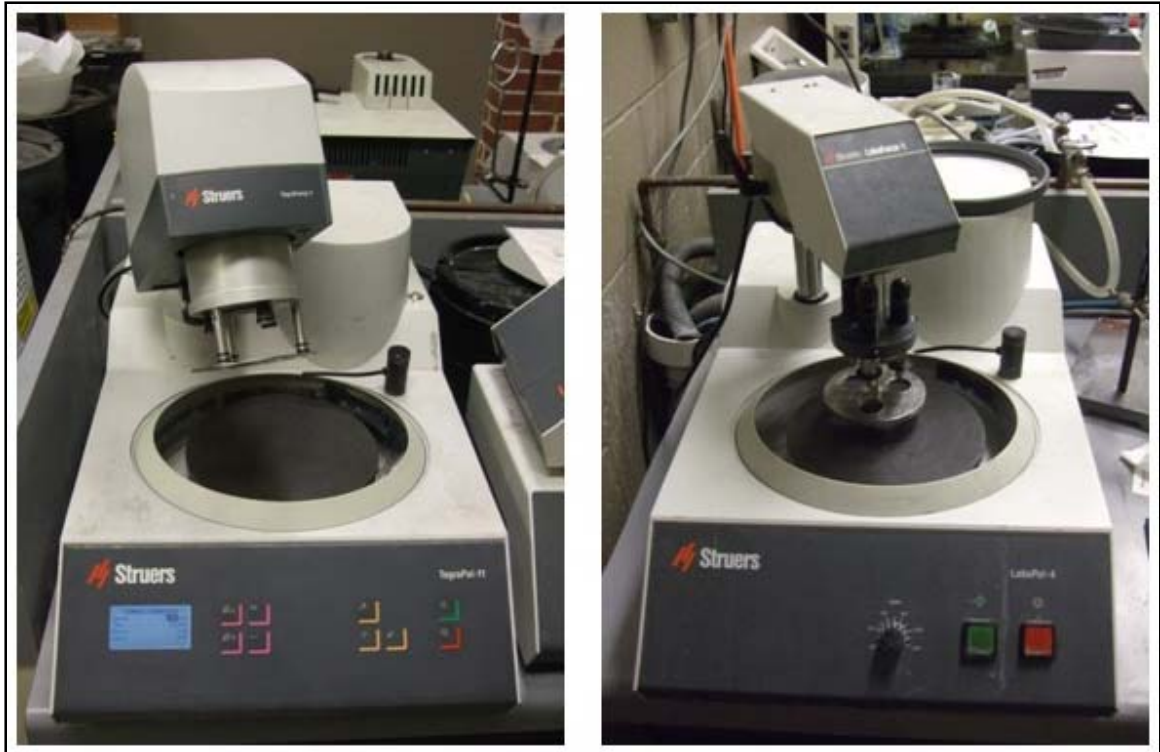
Figure 4.2 The Polishing equipment utilized to prepare samples for analysis. The image on the left represents the Struers LaboPol-11. This is used for the first four steps in polishing. The machine on the right is the Struers LaboPol-4, and it is used in the final stage of polishing.
