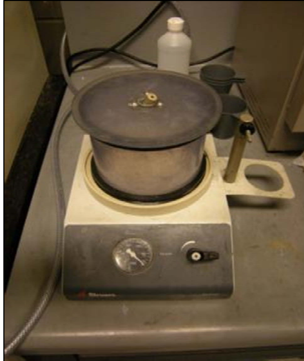
Figure 4.1 Image of the Struers equipment used to cold mount the samples. A vacuum is created inside of the chamber to apply the resin mixture and prevent bubbles (bubbles in the mount can lead to trapped grit later in the polishing stages).
