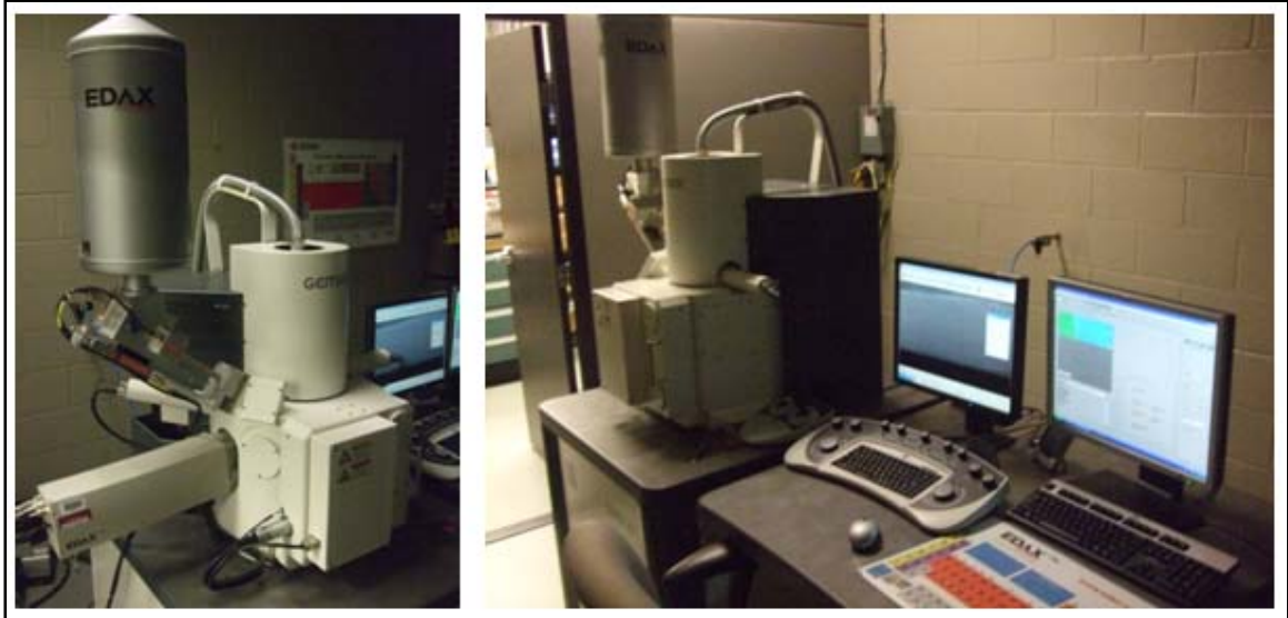
Figure 4.5 The FEG scanning electron microscope is represented on the left. The picture on the right represents the entire setup: FEG SEM, SEM control software, and the OIM data collection software from left to right respectively.
