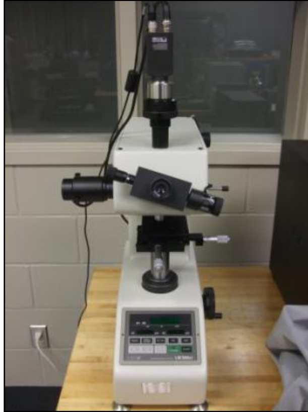
Figure 4.3 The Microhardness indenter used to gather hardness data of the deformed and annealed samples.
