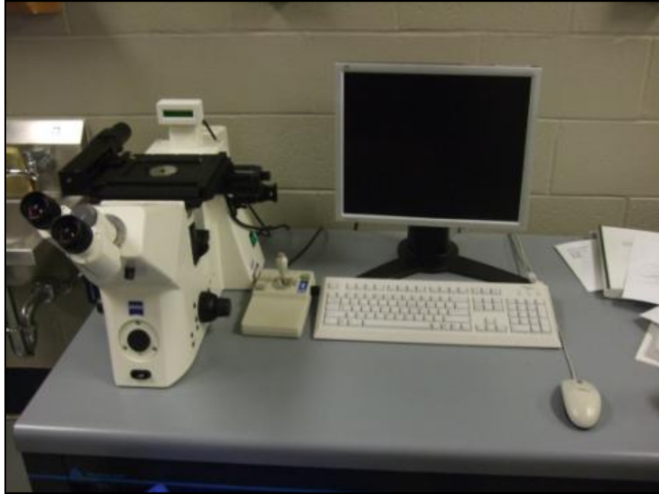
Figure 4.4 Image displaying the system used for optical microscopy. The system includes a Zeiss optical microscope (on the left) and Zeiss image analysis software on the computer represented on the right.
