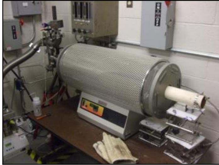
Figure 3.7 Image of the carbolite tube furnace used to anneal samples at the specified times and temperatures. Samples are inserted and extracted through the tube extruding from the right portion of the furnace.
