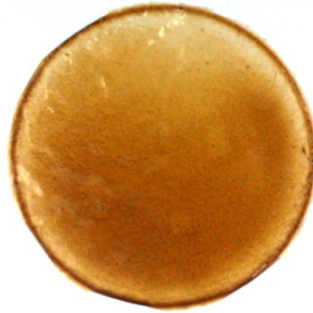
Figure 3.17 Sugarcane bagasse HC-based film.
