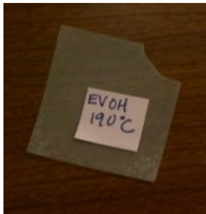
Figure C.6 EVOH film produced at 190° C 4000 lbs. with dried pellets.
