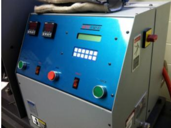
Figure C.2 Picture indicating red switch for powering compression molder.
