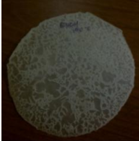
Figure C.5 EVOH film produced at 190° C and 4000 lb f without drying pellets.
