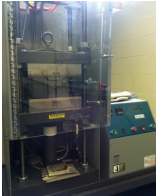
Figure C.4 Carver, Inc. compression molder (model 3893.4PR1A00).
