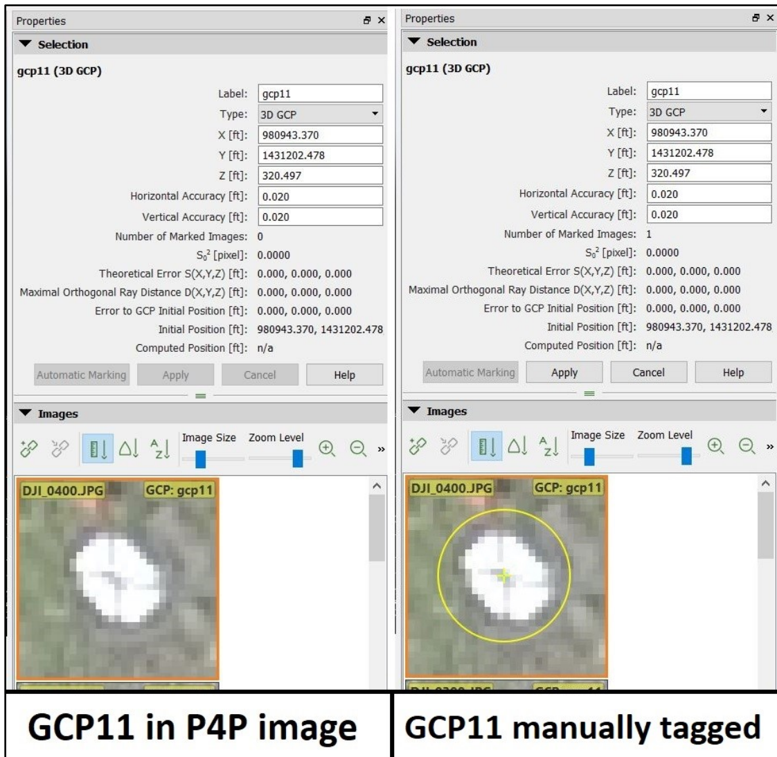
Figure 5.4 Ground Control Point (GCP) Implementation
