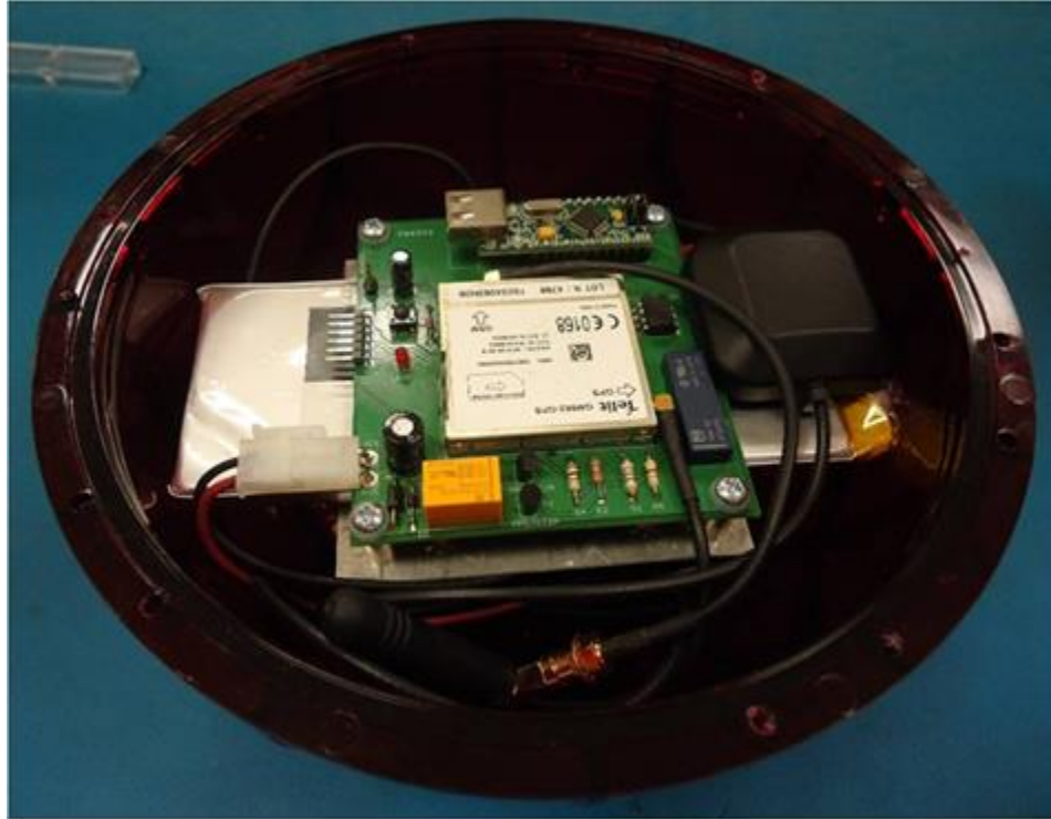
Figure 2.2 The interior circuit board of the GPS drone.
