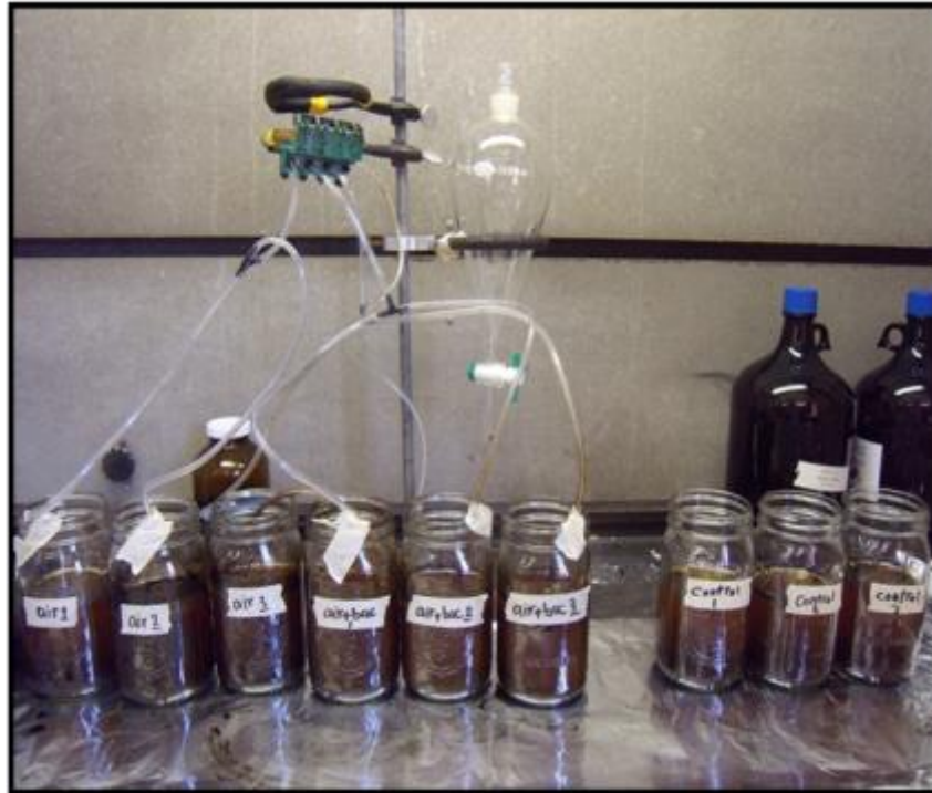
Figure 3 Bio-treatment units (glass canning jars) with sparged air distribution system
