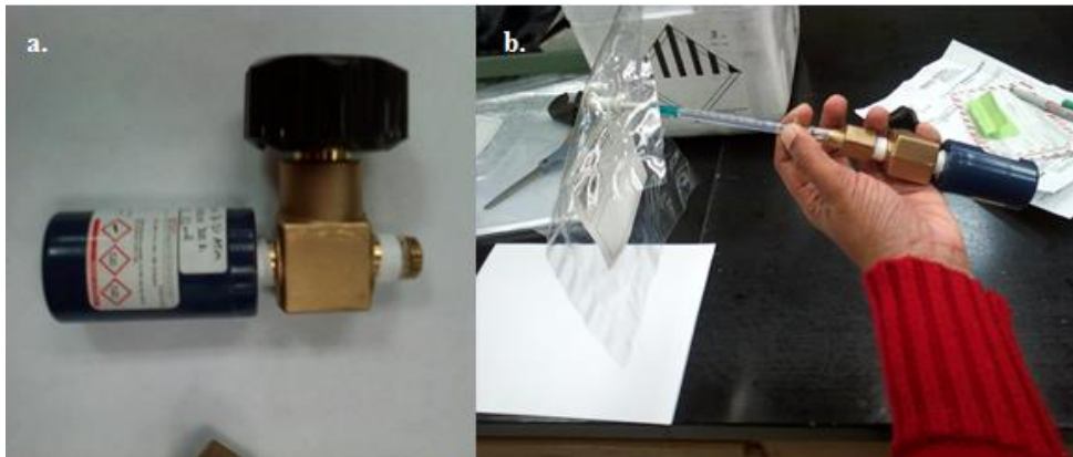
Figure 3.2 ^{15}N_2 isotopic gas at 98 atom% and dilution into 5% using gas sampling bags (a.) ^{15}N_2 isotopic gas (b.) dilution procedure
