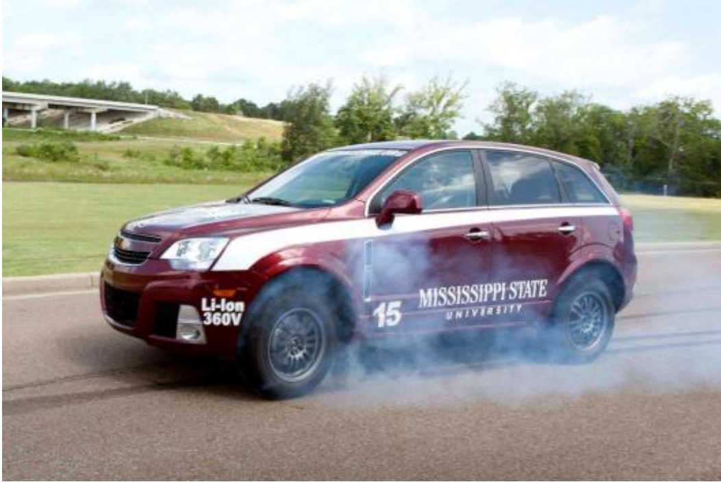
Figure 3.4 Traction control testing on a closed road track in Starkville, MS.
