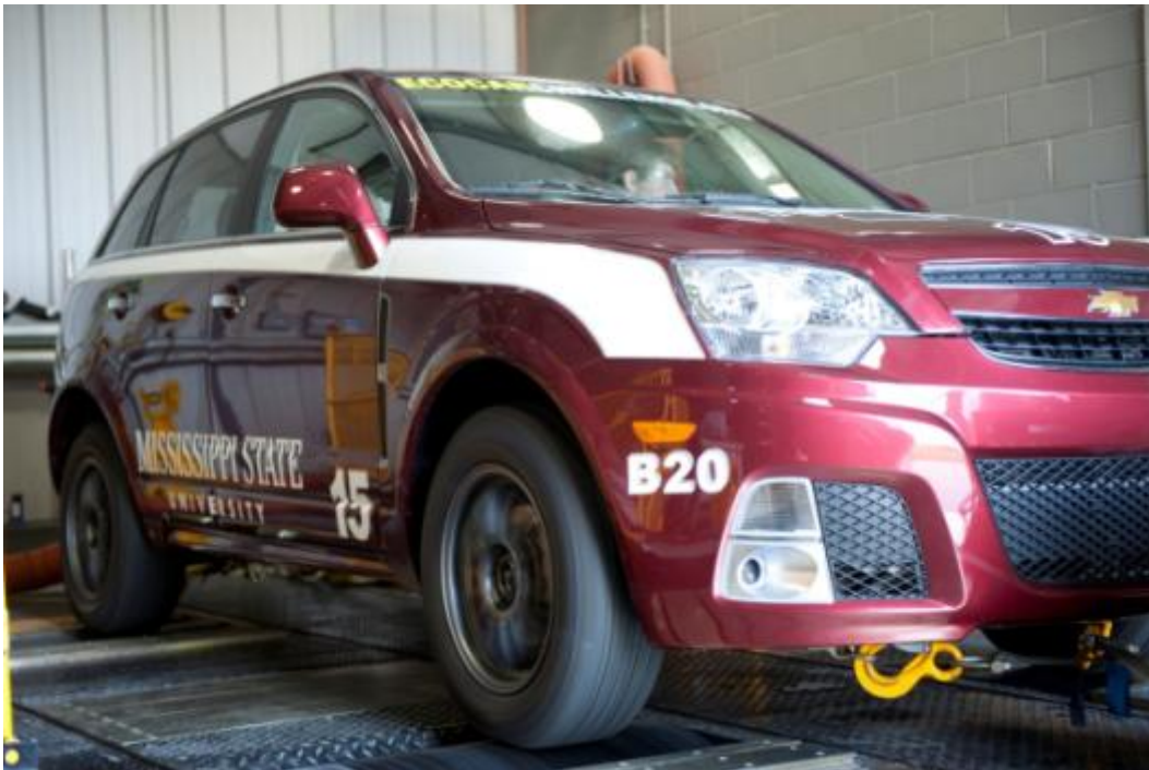
Figure 3.5 Chassis dynamometer testing at Center for Advanced Vehicular Systems (CAVS) in Starkville, MS.
