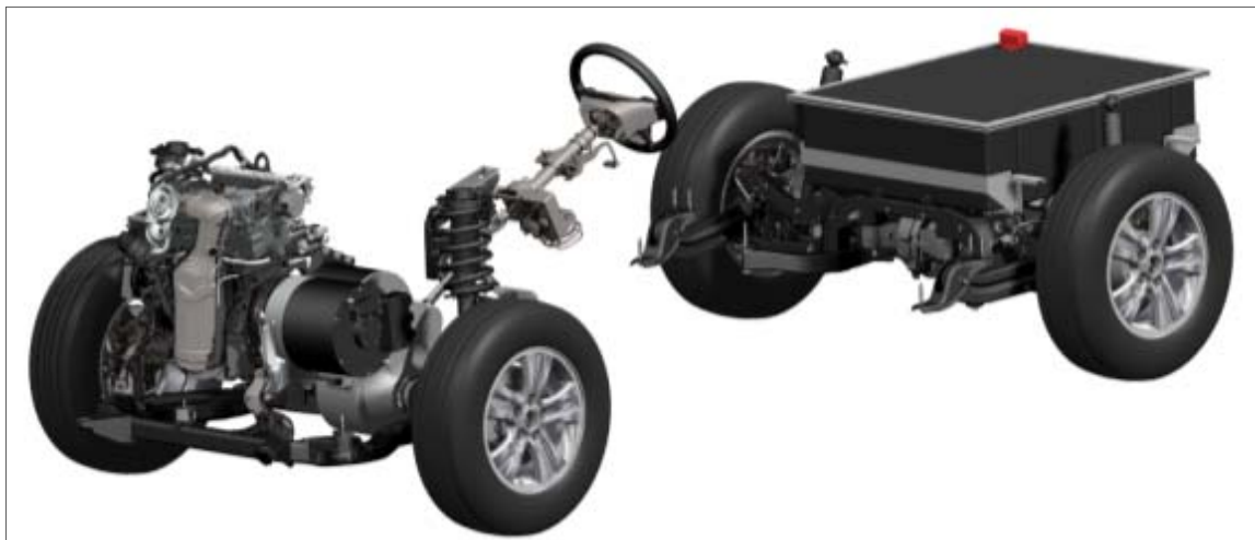
Figure 1.2 EcoCAR vehicle powertrain architecture.
