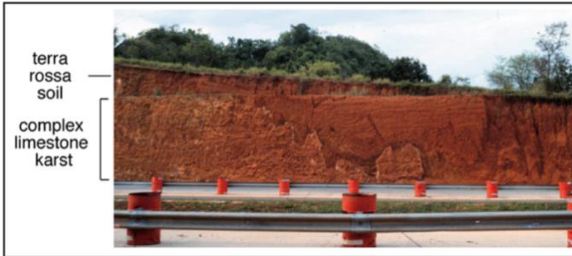
Figure 2.9 This road cut shows cutter-and- pinnacle topography at depth (arrows), which allows for differential compaction if a structure is built on the land surface (i.e. compacting more on the right than on the left).
