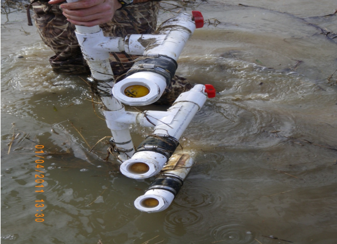
Figure 4.7 Permanent staked samplers situated 200-1200 mm above sediment surface, located at the inflow and immediately downstream of each weir at Terrace Ditch, Yazoo County, MS.
