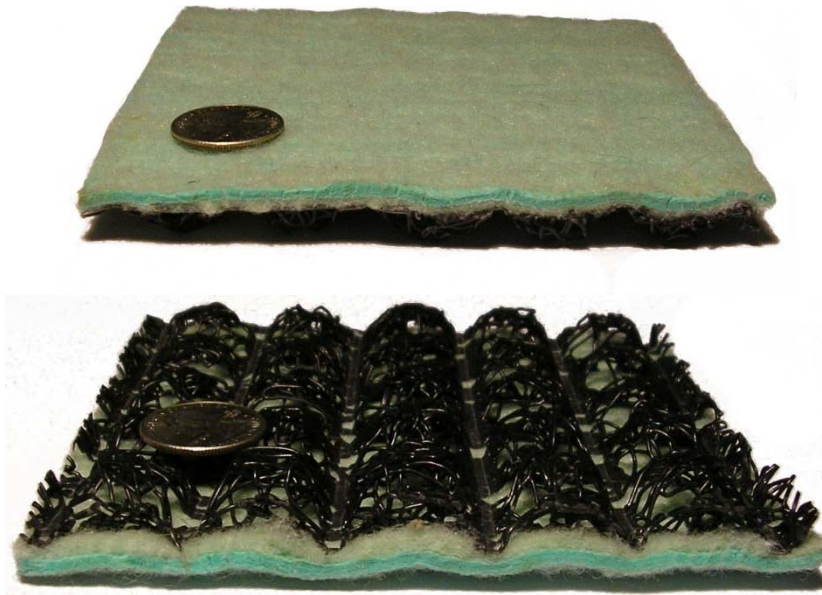
Figure 3.4 Two views of integrated drainage/retention layer ( Enka Retain & Drain 3211 ). Top image shows filter/retention fabric on upper side of product. Lower image shows entangled polypropylene filaments on underside of product.
