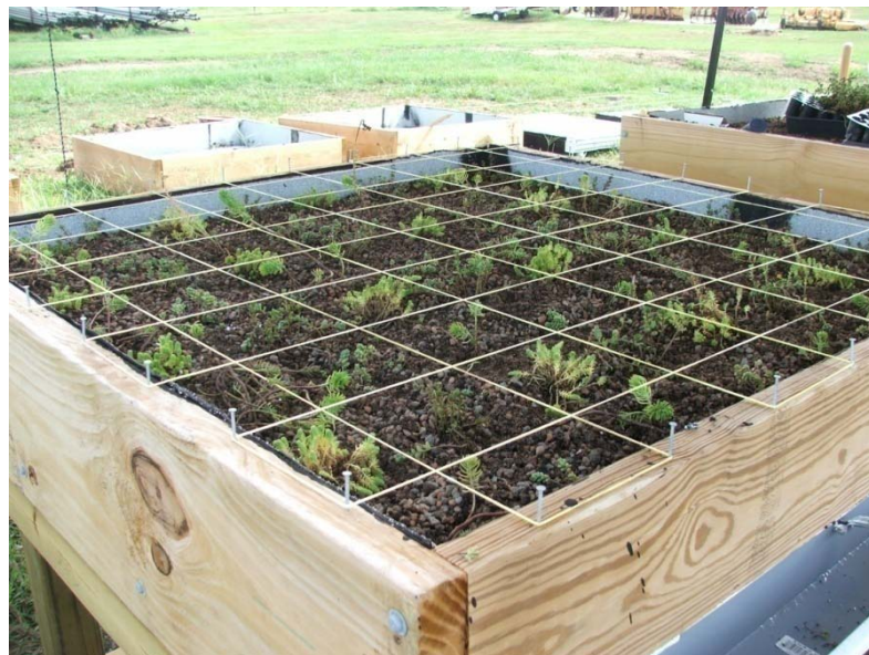
Figure 3.7 View of newly-planted roof platform with 6 in. planting grid.
