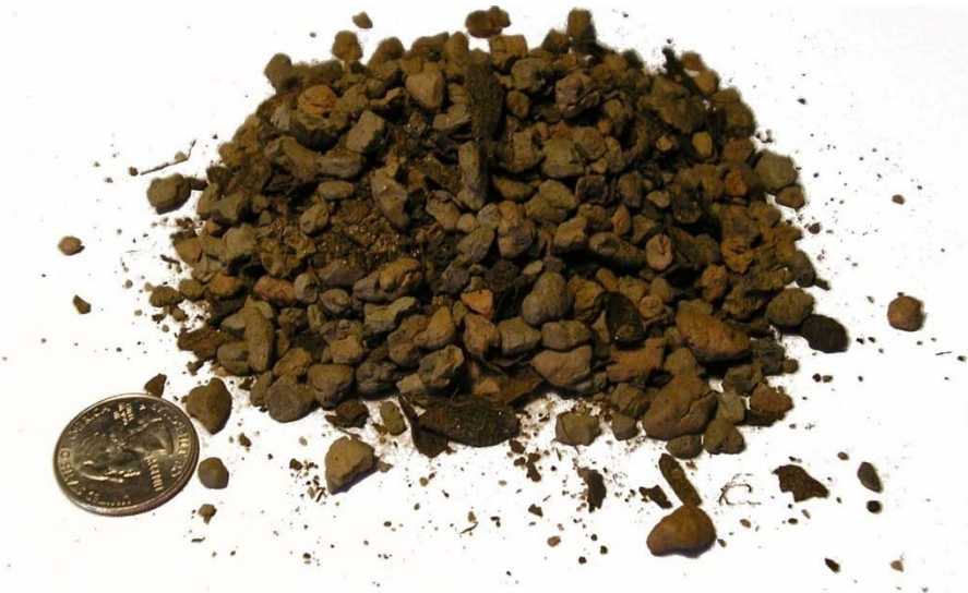
Figure 3.5 Engineered green roof soil ( ERTHHydrocks Lightweight Soil Media-Extensive ). Mix is 80% expanded clay particles, 5% USGS Sand, 15% nutrient-grade compost.
