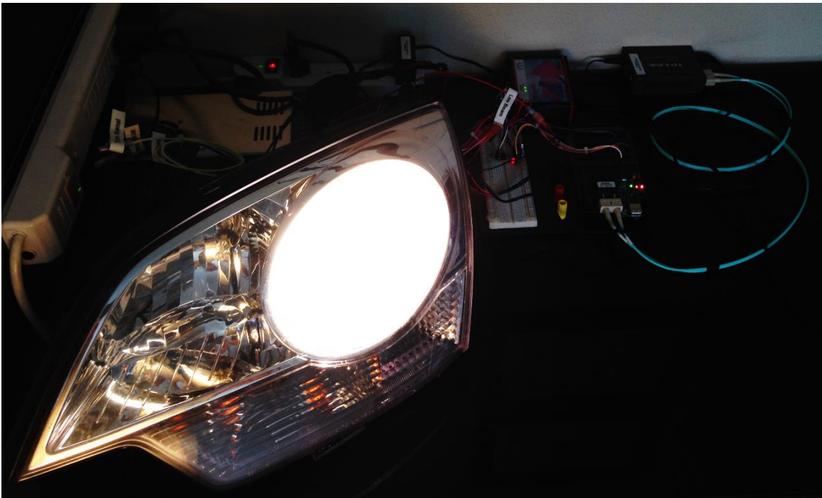
Figure 5.2 Low beam on, controlled from Python GUI
