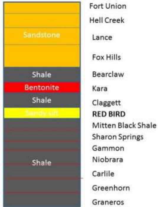
Figure 2.6 Stratigraphic column from west of the Black Hills
