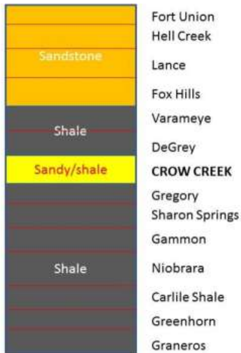
Figure 2.7 Stratigraphic column east of the Black Hills
