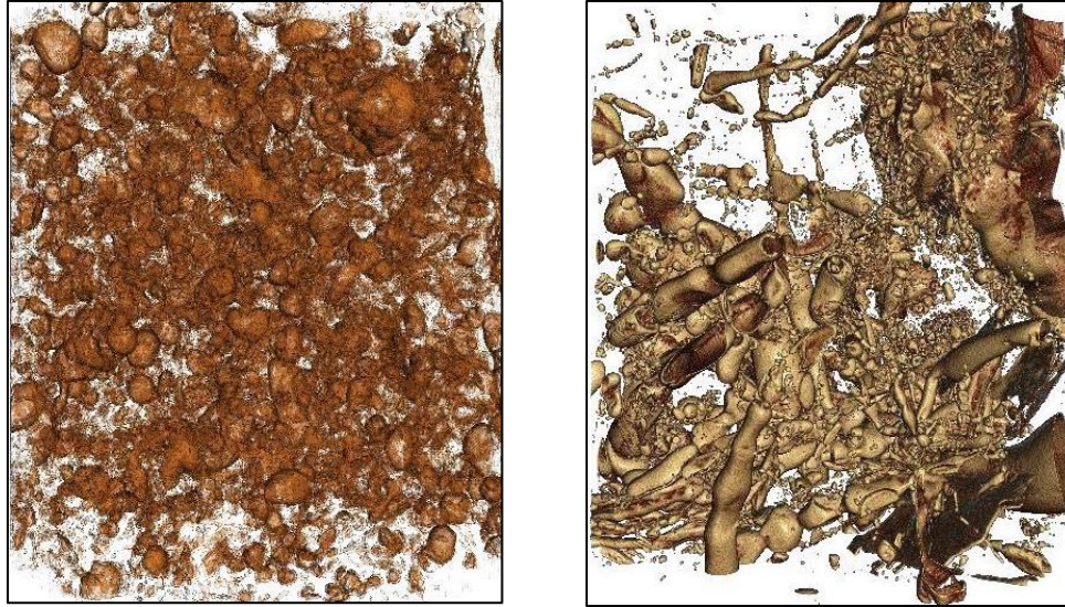
Figure 3.18 3D rendering of scanned area of hybrid resins with the molecular weight of A (left) and W (right)
