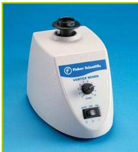
Figure 3.12 Fisher Scientific Vortex Mixer Utilized for Mixing Additives
