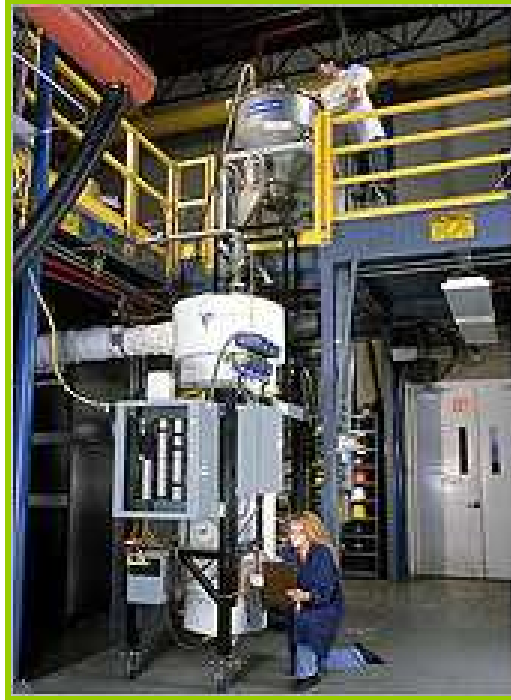
Figure 3.7 A Pictorial View of the National Renewable Energy Laboratory (NREL) Entrained Flow Reactor (Obtained with Permission)
