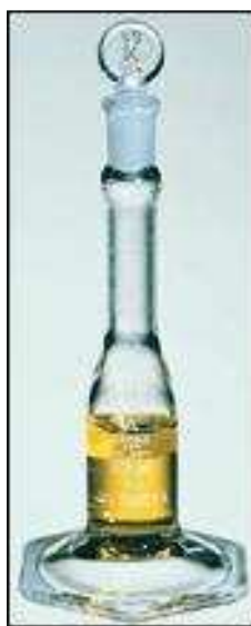
Figure 3.21 Kimax ® Volumetric Flask (Capacity=1 ml) Used for Density Measurements
