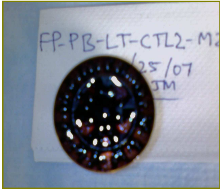
Figure 4.109 Rheometer Spindle Revealing the Sheared Pine Bark Pyrolysis Oil
