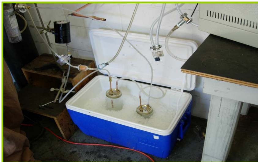
Figure 3.4 Gas Analysis Setup Used with the Mississippi State University (MSU) Small-Scale Auger Reactor System
