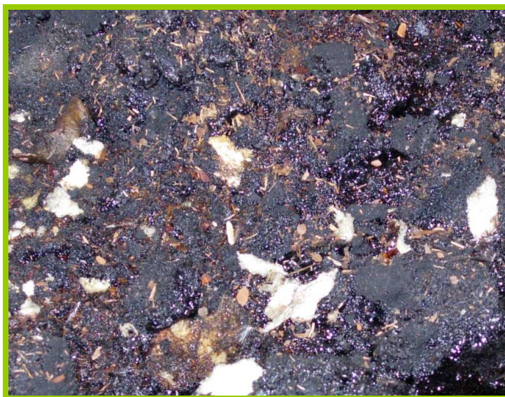
Figure 4.3 Tarry Pyrolyzate Collected from the Mississippi State University Auger Reactor Condensers
