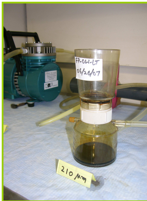
Figure 3.11 Millipore ® Vacuum Filtration Apparatus Used for Pyrolysis Oil Filtration
