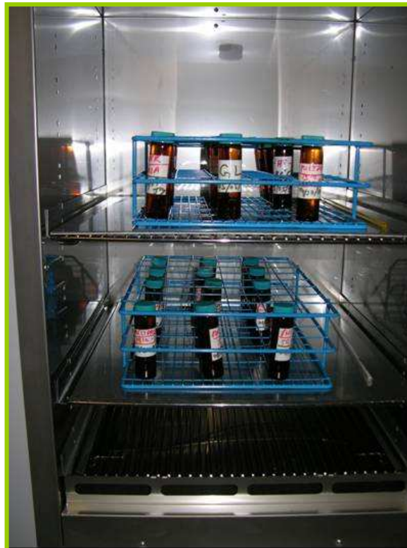
Figure 3.14 Gravity Convection Oven Used for Accelerated ( 80\pm 2^{\circ}\text{C} ) Stability Testing in Phases II-IV
