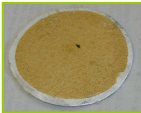
Figure 4.6 Tarry Mass Collected During Gas Analysis of Mississippi State University Pine Bark-Low Temperature-Fast Residence (PB-LT-FR) Pyrolysis Oil
