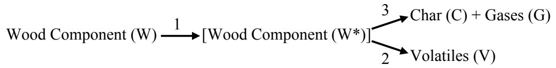
Figure 2.7 Lumped 3-Step Kinetic Model of Wood Pyrolysis (Shafizadeh, 1982)
