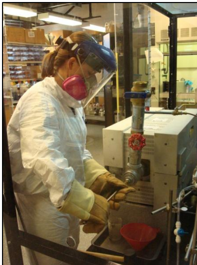
Figure 3.33 Pushing CCA-Treated Wood into the Batch Pyrolysis Reactor during Phase III of the CCA-Treated Wood Waste Study
