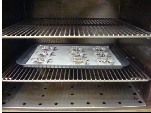
Figure 3.13 Sawdust Samples in Forced Air Oven during Moisture Content Determination of CCA-Treated Wood Waste
