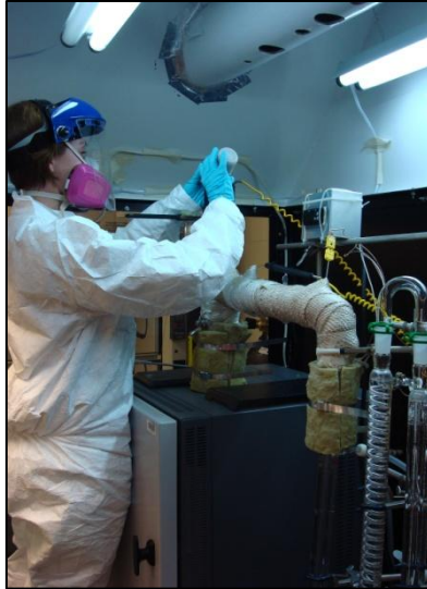
Figure 3.21 Loading CCA-Treated Wood into the Bench Pyrolysis Reactor during Phase II of the CCA-Treated Wood Waste Study
