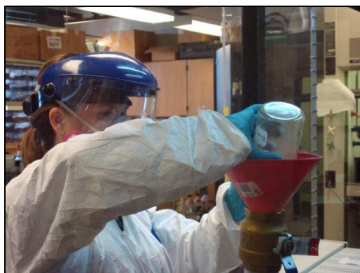
Figure 3.32 Loading CCA-Treated Wood into the Batch Pyrolysis Reactor during Phase III of the CCA-Treated Wood Waste Study
