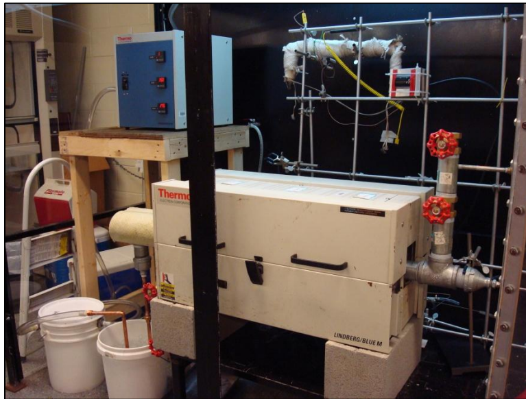
Figure 3.25 Batch Pyrolysis System Used to Generate Char for EK Experiments in the CCA-Treated Wood Waste Study
