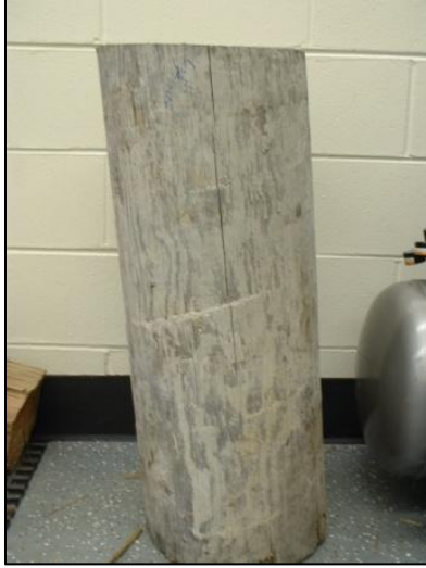
Figure 3.3 4 Foot Section of the CCA-treated Wood Utility Pole
