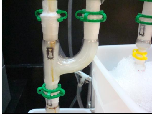
Figure 3.23 Observed Pyrolysis Vapor in a Condenser Outlet of the Bench Pyrolysis System during Phase II of the CCA-Treated Wood Waste Study
