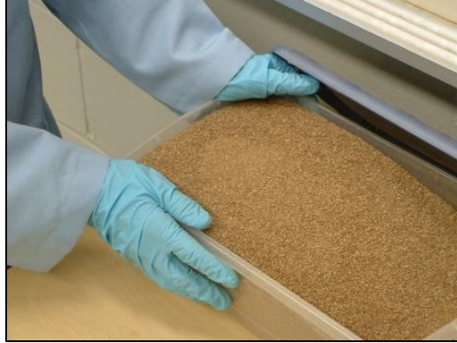
Figure 3.5 CCA-Treated Wood Sawdust Used in All Experiments of this Study
