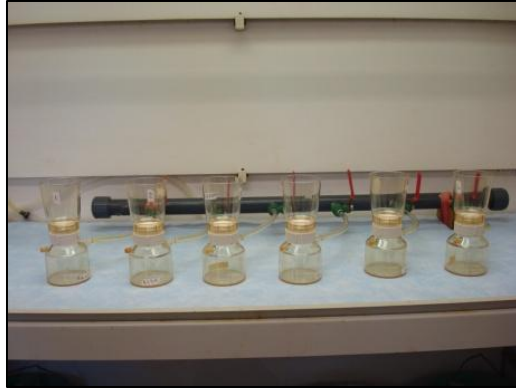
Figure 3.9 Vacuum Filtration Apparatus Set-up Utilized Throughout CCA-Treated Wood Study
