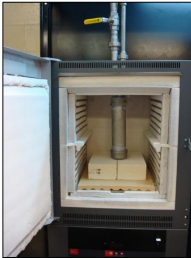
Figure 3.17 Bench Pyrolysis Reactor of the CCA-Treated Wood Waste Study – Without Insulation
