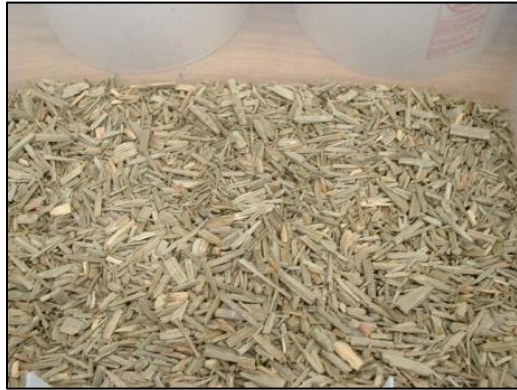
Figure 3.4 Chipped Pieces of the CCA-treated Wood Utility Pole
