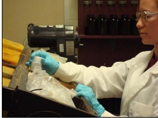
Figure 3.11 Placing TCLP Samples in Tumbler for CCA-Treated Wood Waste Characterization Study – Close View
