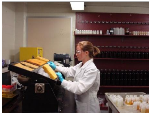
Figure 3.10 Placing TCLP Samples in Tumbler for CCA-Treated Wood Waste Characterization Study
