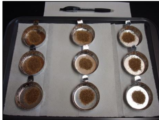
Figure 3.12 Sawdust Samples in Metal Sample Tins for Moisture Content Determination of CCA-Treated Wood Waste
