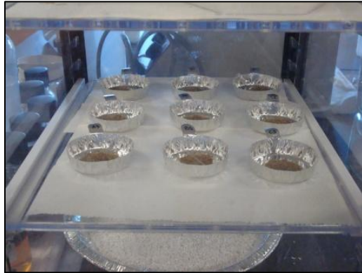
Figure 3.14 Sawdust Samples in Dessicator during Moisture Content Determination of CCA-Treated Wood Waste
