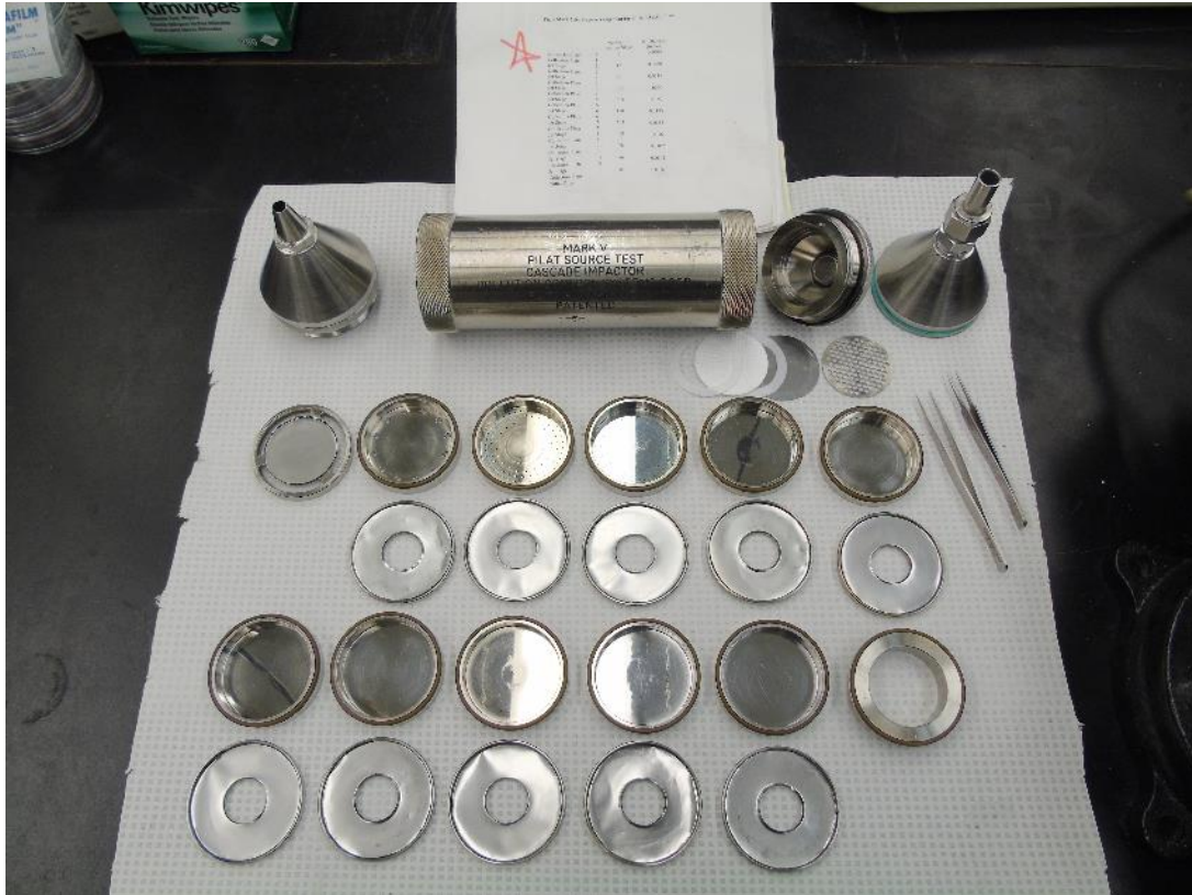
Figure 3.5 Jet stages and collection plates of the Pilat impactor.
