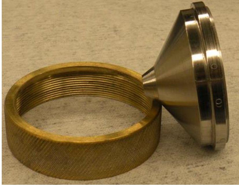
Figure 2.2 Isokinetic sampling nozzle and knurled retaining collar of the sampler.
