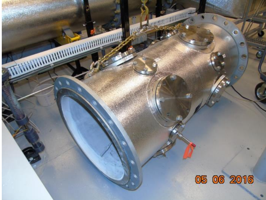
Figure 2.23 Modified duct section for the isokinetic samplers.
