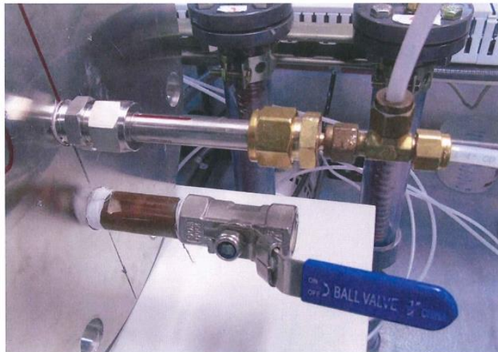
Figure 4. Vacuum tubing attached to end of sampler.
