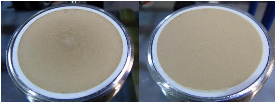
Figure 2.18 Loading pattern using original vs. revised sampling nozzle design.
