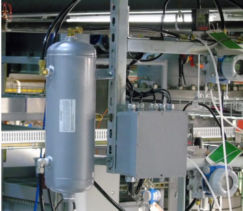
Figure 2.8 Ballast tank for the isokinetic samplers.
