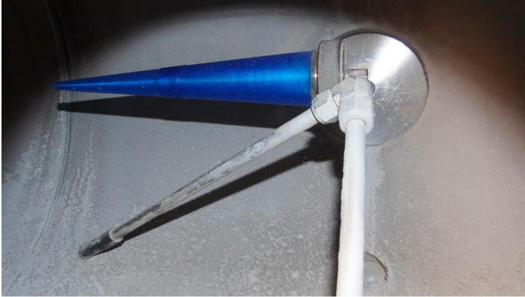
Figure 2.16 Prototype nozzle design installed onto isokinetic sampler base.
