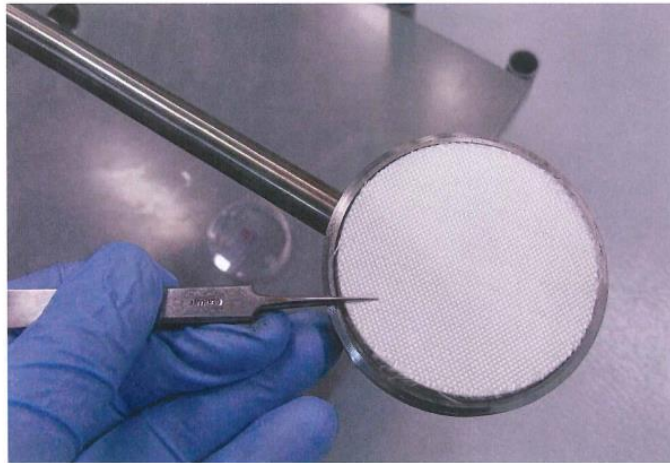
Figure 1. Installing in-duct coupon on sampler
