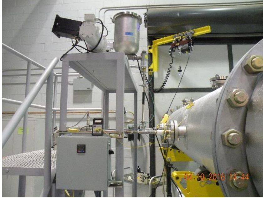
Figure 3.1 K-Tron powder feeder used for test dust generation on the RLSTS.
