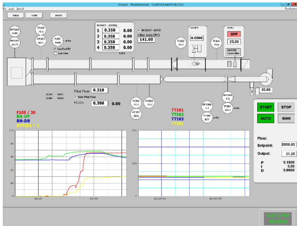
Figure 2.13 RLSTS and isokinetic sampler touchscreen control interface on the SCADA.
