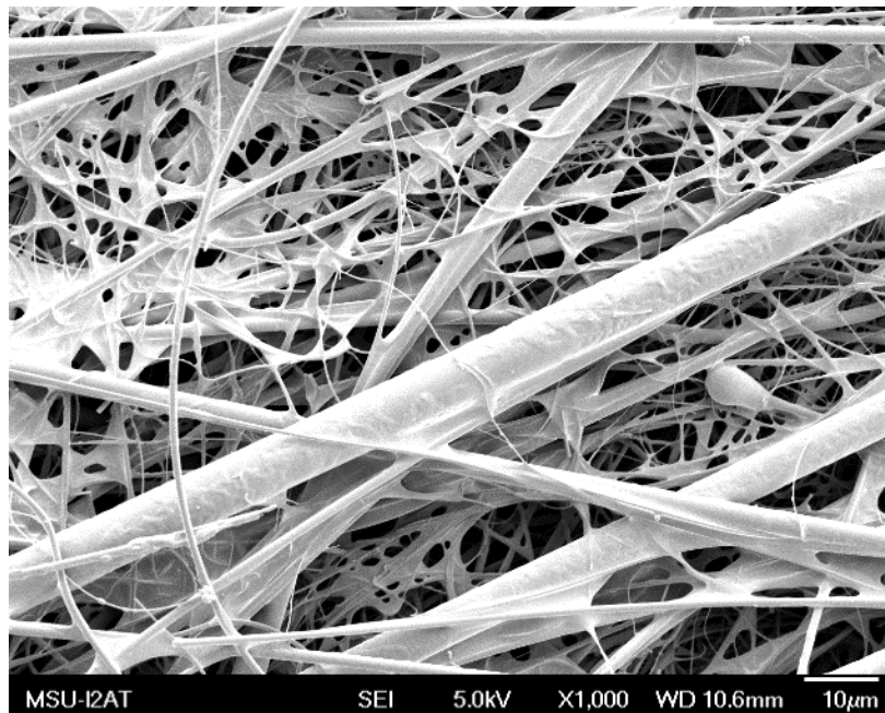
Figure 4.35 SEM image of fiber sizing at x1000 magnification.
