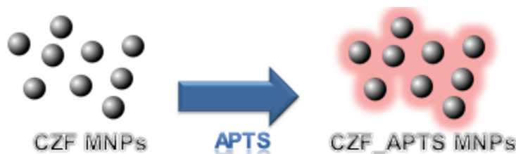
Figure 3.5 Surface modification of CZF nanoparticle to CZF-APTES
