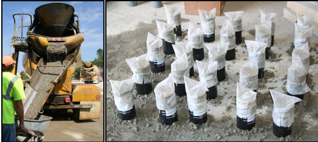
a) Concrete Sampling b) Field Concrete Specimens
