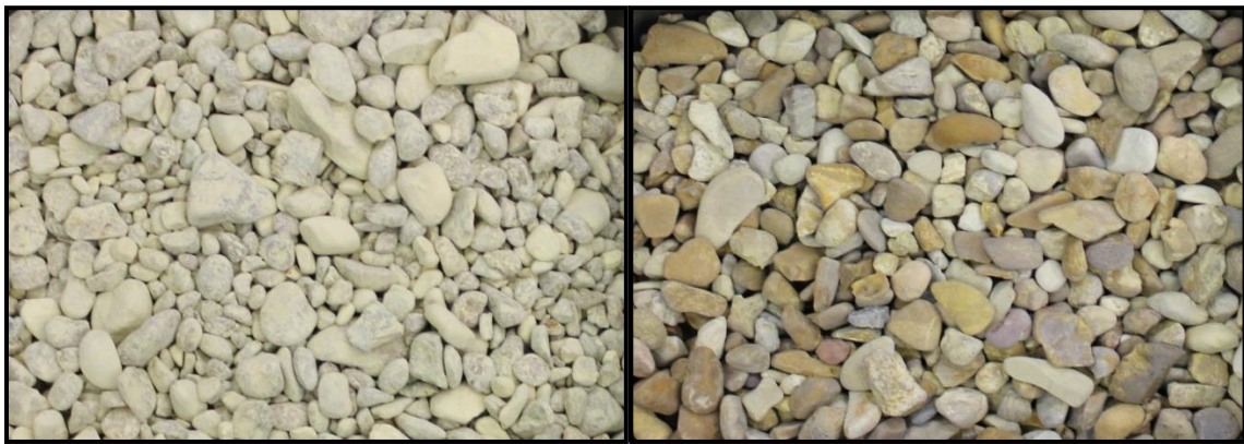
a) Unwashed Sample (Fines of Around 1%) b) Post-Washing Sample (Fines Less Than 1%)
