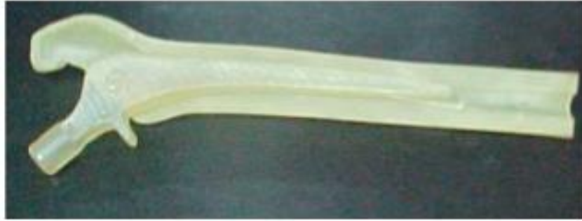
Figure 5.4 Fit check of rapid prototyping part for hip prosthesis
