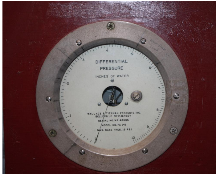
Figure 2.3 Differential Pressure Gage.
