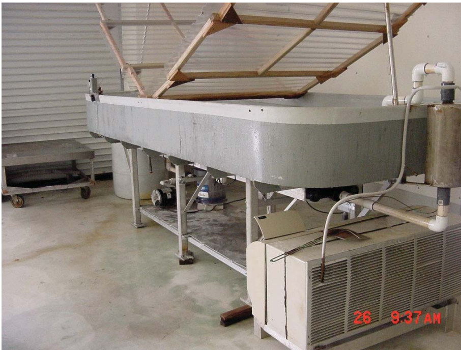
Figure 1. Depuration tank design (Pascagoula, MS)
