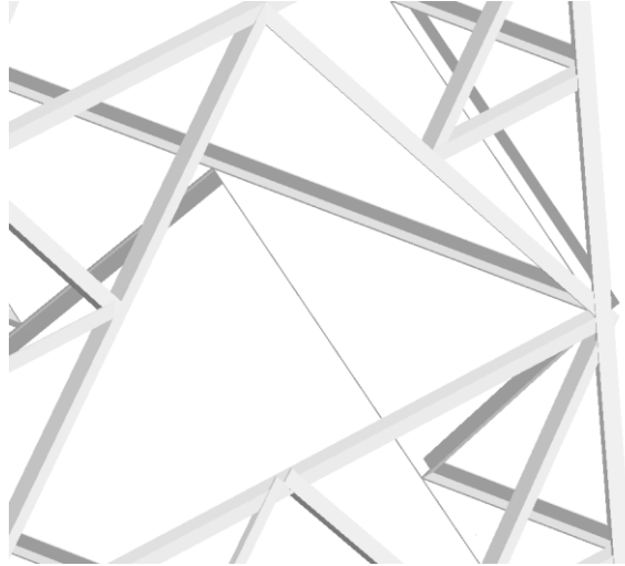
Figure 4.3 L-beams structures within the cell tower design.
