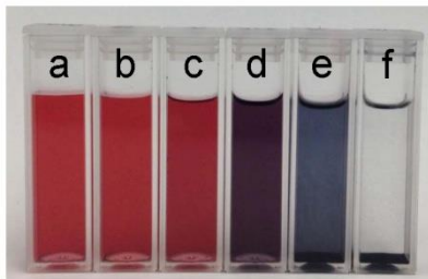
Figure 2.13 Photograph of the AuNP in the water:ethanol cosolvents where the % volume of ethanol in the cuvettes (a) to (f) varies from 0%, 13.3%, 26.7%, 40.0%, 53.3%, and 66.7% , respectively.
