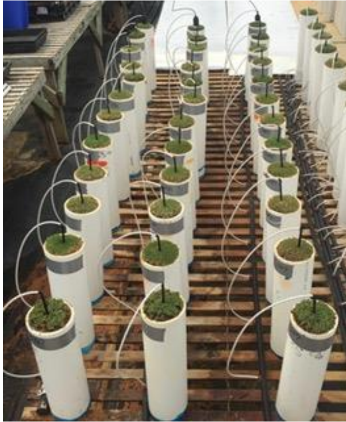
Figure B.1 Left: 0.31 \text{ m}^3 \text{ m}^{-3} Regimen. Middle: 0.15 \text{ m}^3 \text{ m}^{-3} Regimen. Right: 0.05 \text{ m}^3 \text{ m}^{-3} Regimen.
