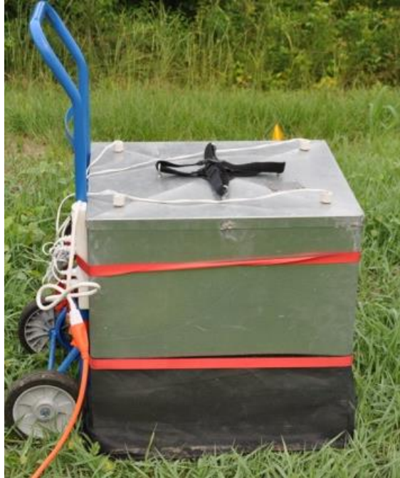
Figure 3.3 The light box used in conjunction with a digital camera to capture photographs for digital image analysis of percent vegetative coverage.
