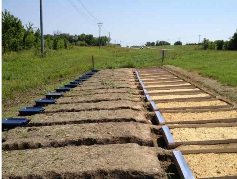
Figure 3.1 Runoff frame and collection container arrangement used for Experiment I and II. Experimental area locations differed between experiments and between years for each experiment.
