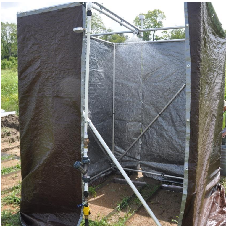
Figure 3.2 The Tlaloc 3000 rainfall simulator (Joern's Inc., West Lafayette, IN) used during Experiment I and II in 2011 and 2012.
