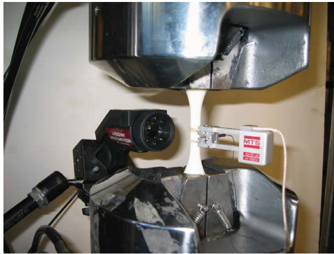
Figure 8 An Acrylonitrile Butadiene Styrene copolymer cylindrical dog-bone shaped fatigue specimen mounted in an MTS 810 servo-hydraulic load frame with an MTS model 634.31F-25 axial extensometer for strain-control tests while an Optris Laser thermometer monitored temperature generation.
