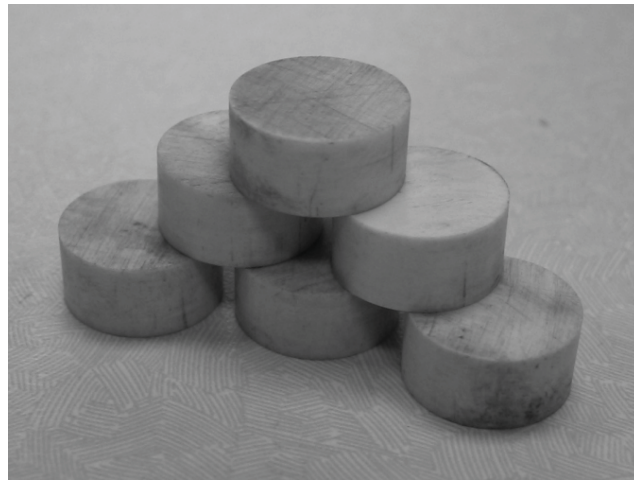
Figure 7 Cylindrical compression specimens with a 12.7 mm diameter and a 1:2 length/diameter ratio were used for monotonic compression tests (shown prior to polishing).
