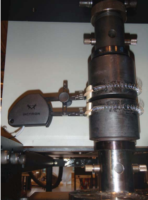
Figure 6 The experimental setup used for monotonic compression tests using an Instron 8850 load frame and an Instron 2630-110 extensometer.
