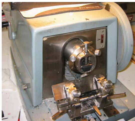
Figure 1 A microtome was used to cut Acrylonitrile Butadiene Styrene copolymer specimens to approximately 5 \mu\text{m} thick films for Fourier Transform Infrared Spectroscopy experiments.
