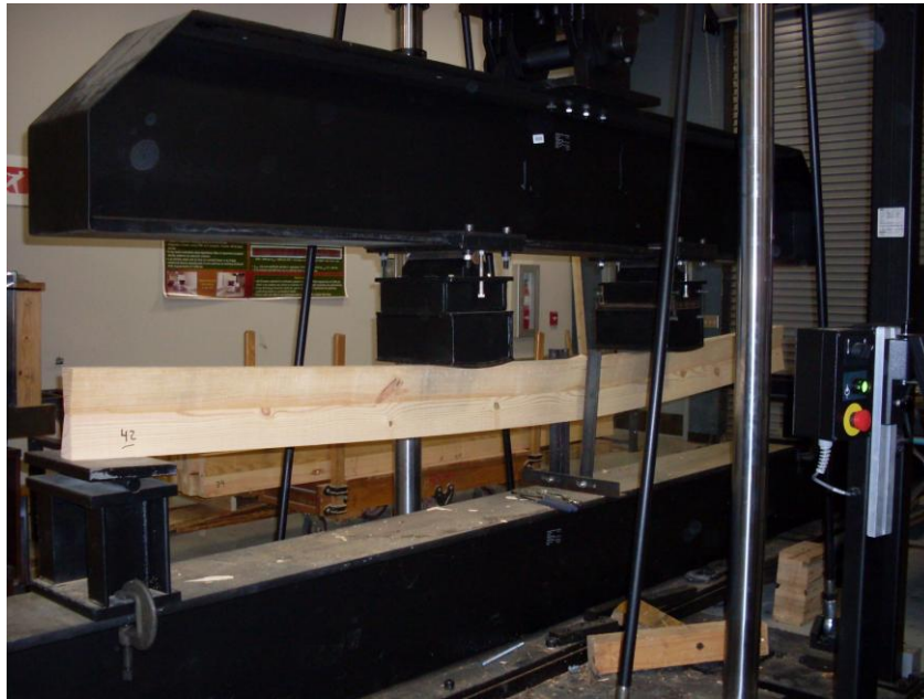
Figure 4.10 Bowtie-Beam has high elasticity property
