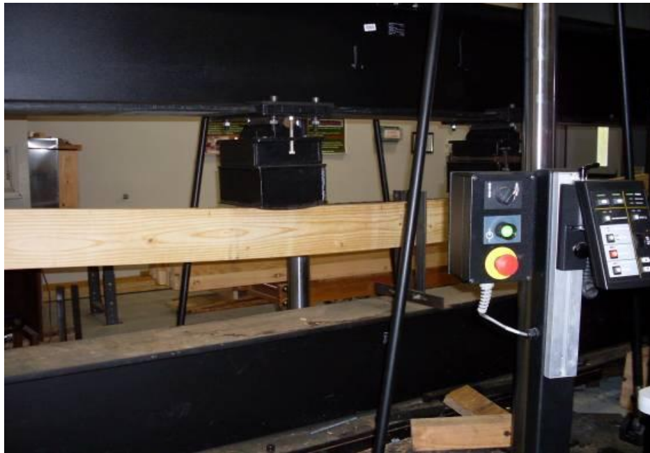
Figure 3.15 Mechanical testing of solid sawn beams
