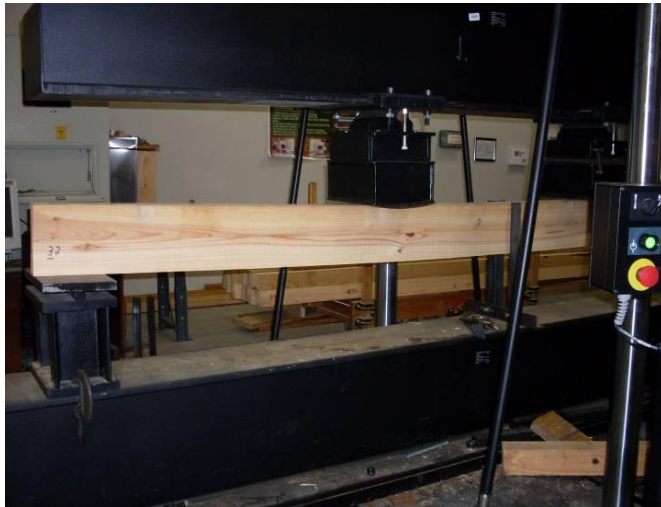
Figure 3.16 Bowtie-Beam mechanical test
