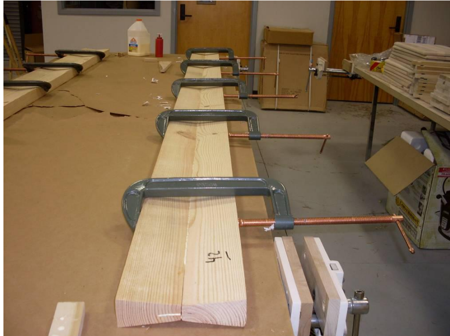
Figure 3.11 Bowtie-Beams during clamping and ambient temperature curing
