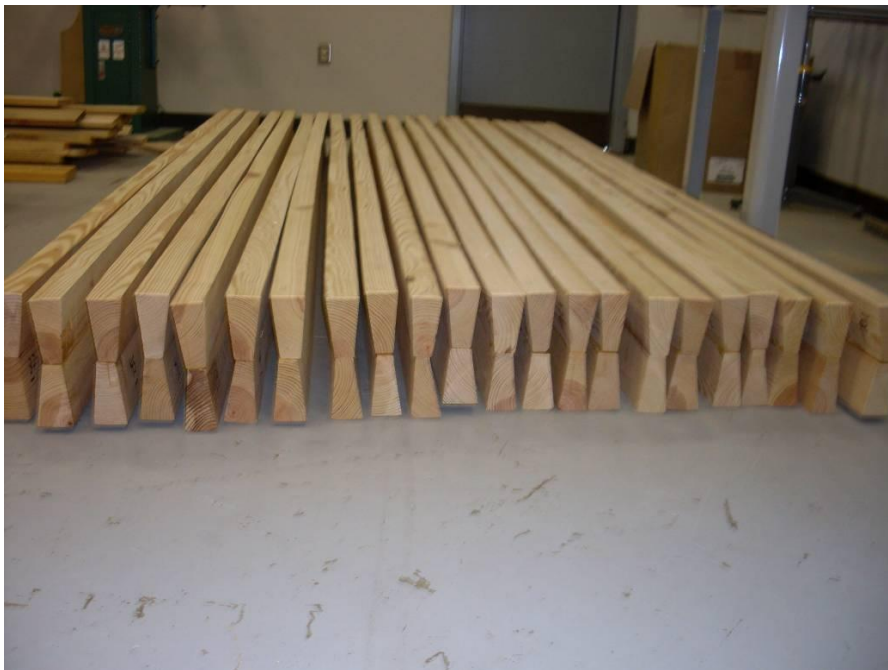
Figure 3.13 The completed 22 Bowtie-Beams
