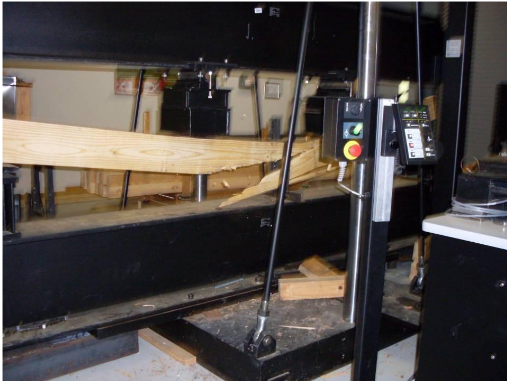
Figure 3.18 Regular beam failure mode
