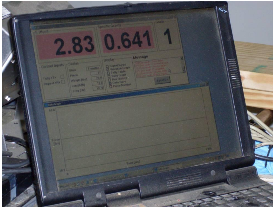
Figure 3.8 E-computer monitor shows the strength and the density
