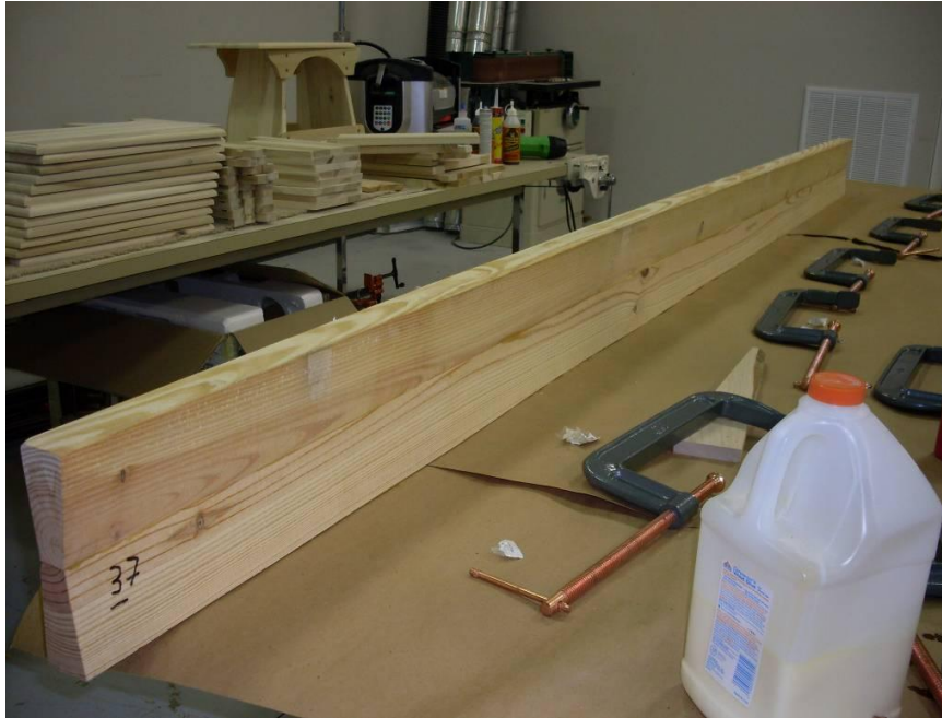
Figure 3.12 The Bowtie-Beam immediately after the glue was cured and the clamps were removed
