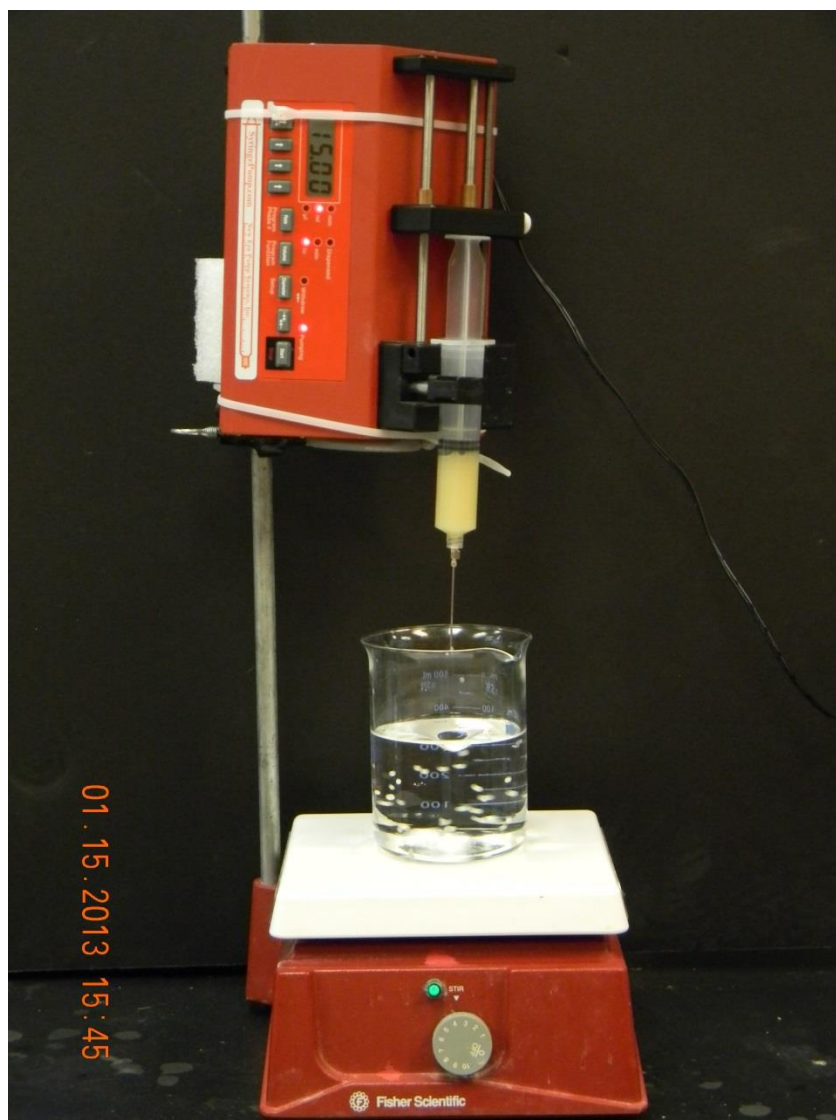
Figure 2.3 Chitosan calcium phosphate solution dripping drop wise into a magnetically stirring precipitate bath at a rate of 15ml per hour.
