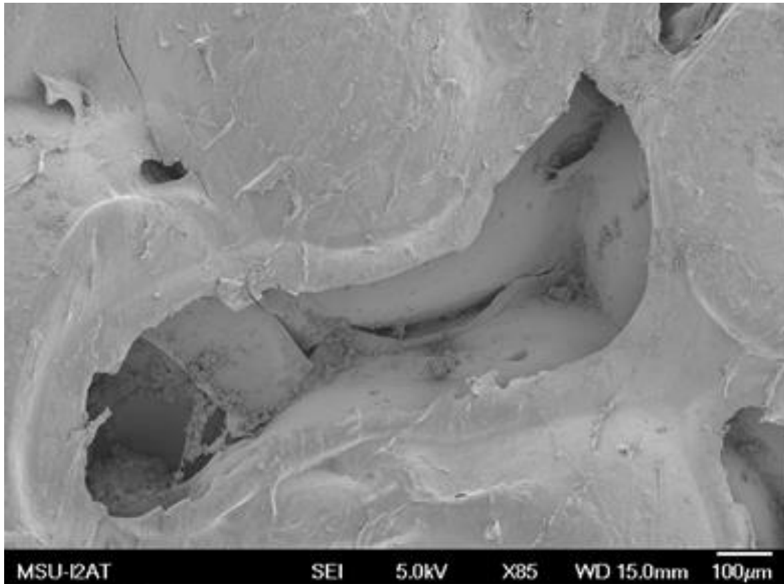
Figure 3.3 Scanning electron micrographs showing the presence of thin sheet of porcine bone marrow mesenchymal stem cells on top of CHI-CaP beads created using approach # 1 (85X).
