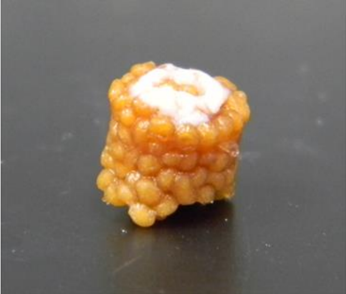
Figure 3.5 Neo cartilage like tissue formed on composite CHI-CaP scaffolds
