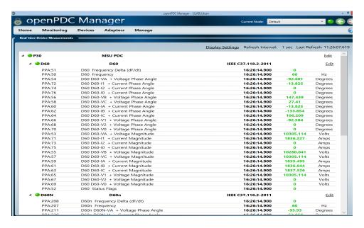
Figure 3.2 Actual measurements from GE D60
