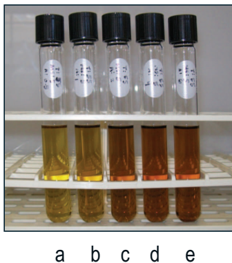
Figure 3.4 Biodiesel dissolved in n -hexane from the in situ transesterification of activated sludge; 55°C, 5 mL methanol/g sludge, a: 0.5%, b: 1.0%, c: 2.0%, d: 4.0% and e: 6.0% H 2 SO 4 .
