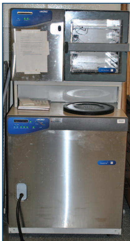
Figure B.6 Freezone 6 Bulk Tray Freeze dry system (Labconco, Kansas City, MO, U.S.A.).
