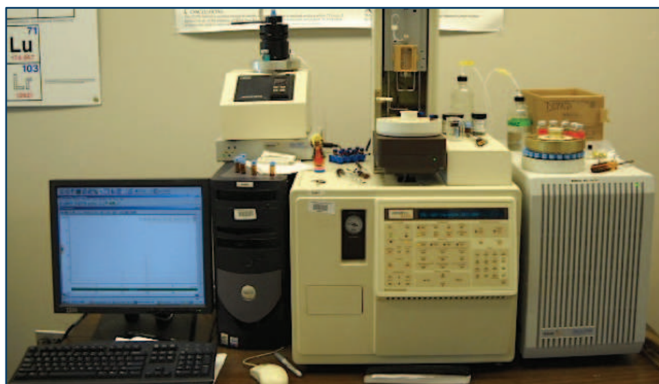
Figure B.18 Varian 3400 GC equipped with a Saturn 2000 ion-trap mass spectrometer (GC-MS) (Varian Inc., Palo Alto, CA, U.S.A.).
