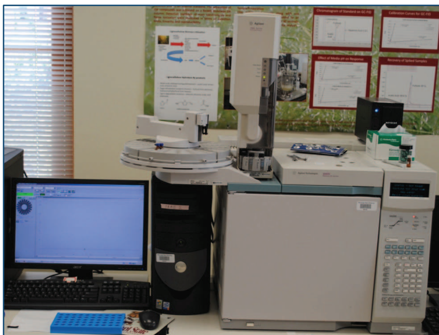
Figure B.16 Agilent 6890N gas chromatograph equipped with flame ionization detector (Agilent, Santa Clara, CA, U.S.A.).
