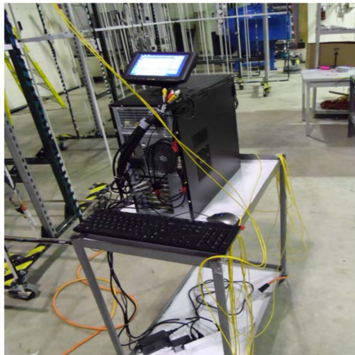
Figure 5.8 The multi-functional portable FLRD control device.
