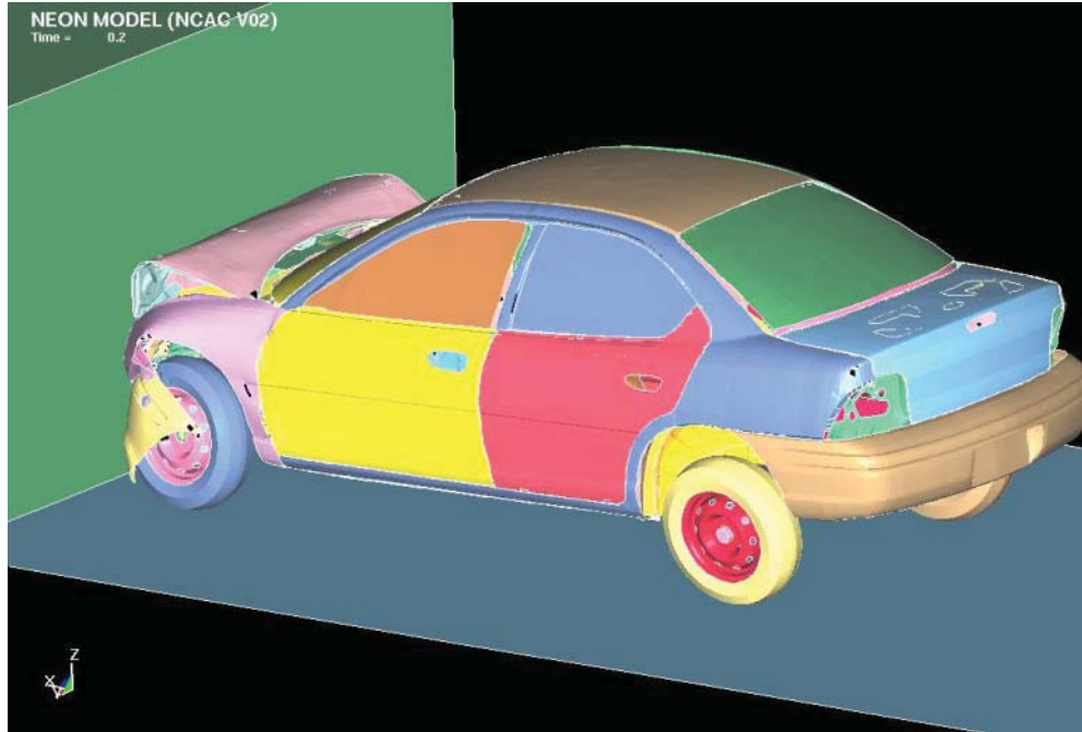
Figure 8 Finite Element Method simulation describing the impact of an automobile with a rigid object; From (Rahmm Tech)
