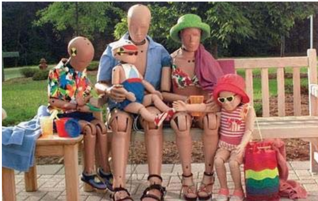
Figure 6 Family of Hybrid III Dummies designed to consider the entire general public; From [15]
