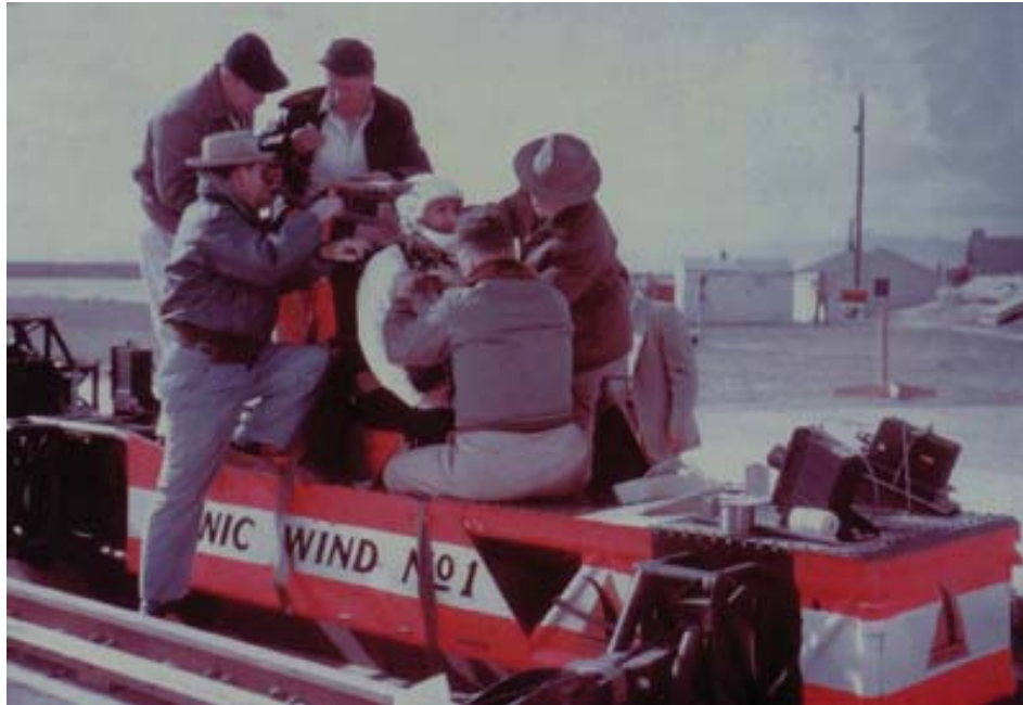
Figure 2 Example of Volunteer Testing in High Impact Scenario; Colonel John Paul Stapp in a rocket sled; from [6]
