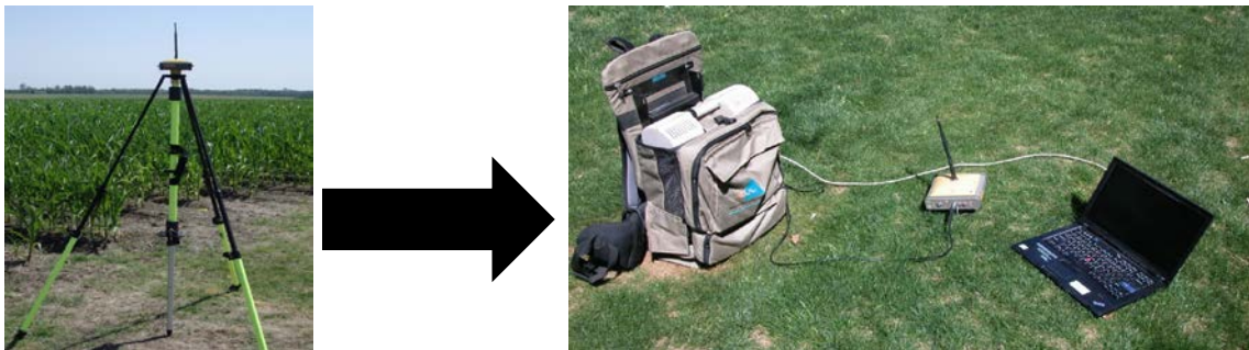
Figure 2.1 Topcon HiPer Lite Plus RTK GPS and Fieldspec Pro handheld spectroradiometer integration.
