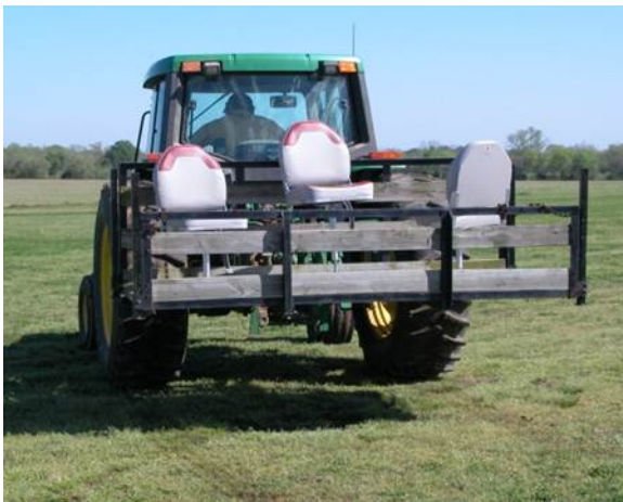
Figure 2.2 Tractor mounted platform for on-the-go data collection.
