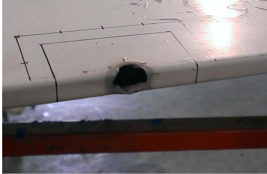
Figure 1.4 Typical lightning damage to Bombardier DHC 8-102.
