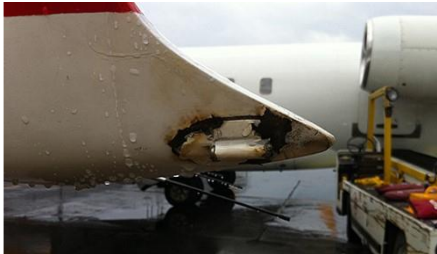
Figure 1.5 Typical lightning damage to Bombardier RJ 100.
