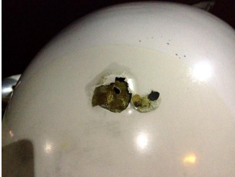
Figure 1.3 Lightning damage to the composite radome of Beechcraft Model 99 [30].
