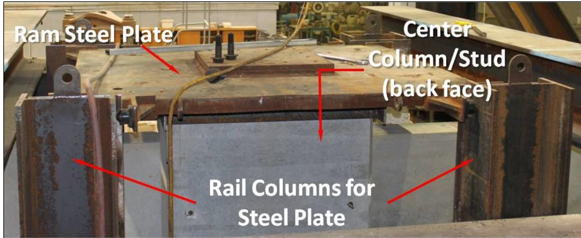
Figure 3.10 Ram steel plate and rail columns of reaction structure
