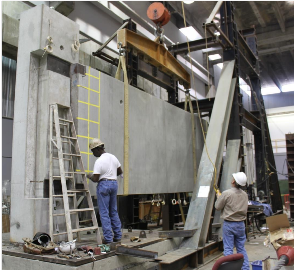
Figure 3.7 Assembly of spandrel beams into the moment frame
